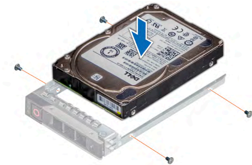
Figure 54. Installing a drive into the drive carrier
