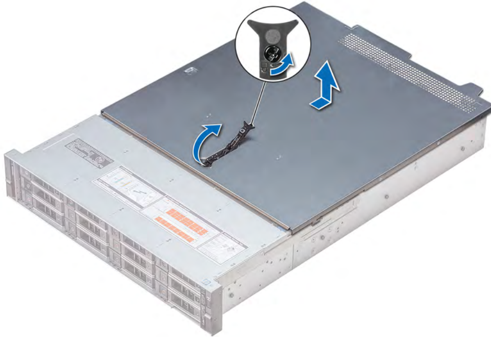
Figure 25. Removing the system cover
