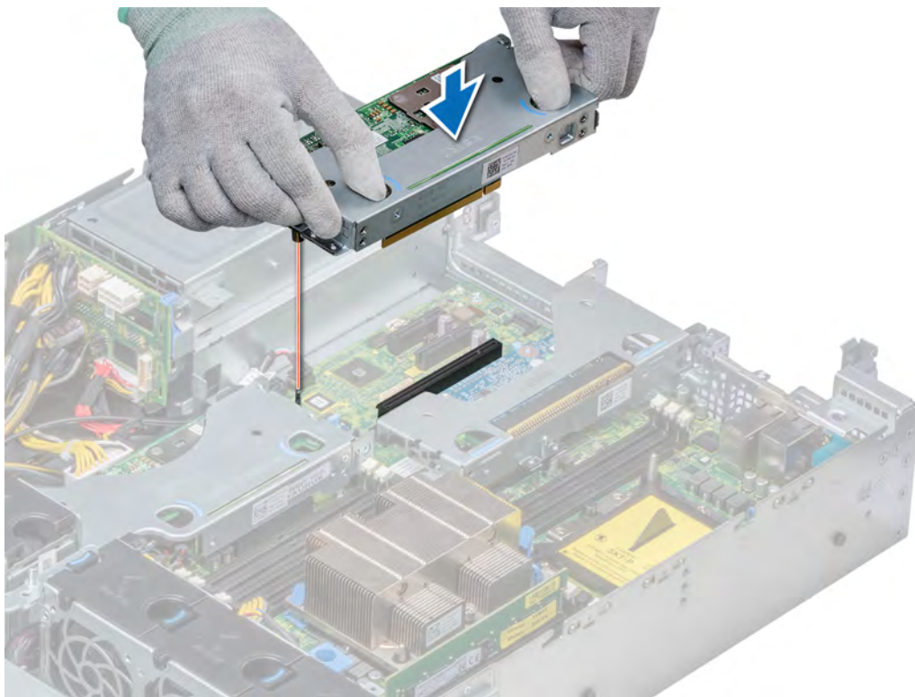
Figure 86. Installing low profile riser left
