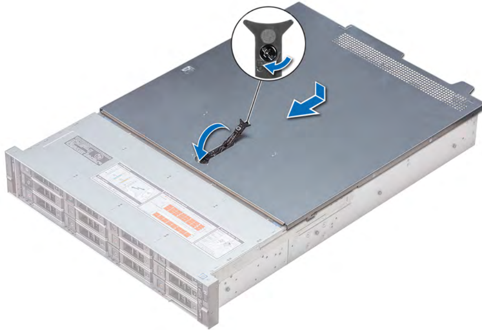
Figure 26. Installing system cover
