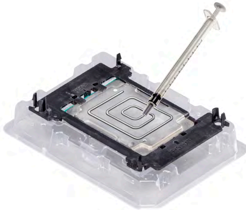
Figure 62. Applying thermal grease on top of the processor
