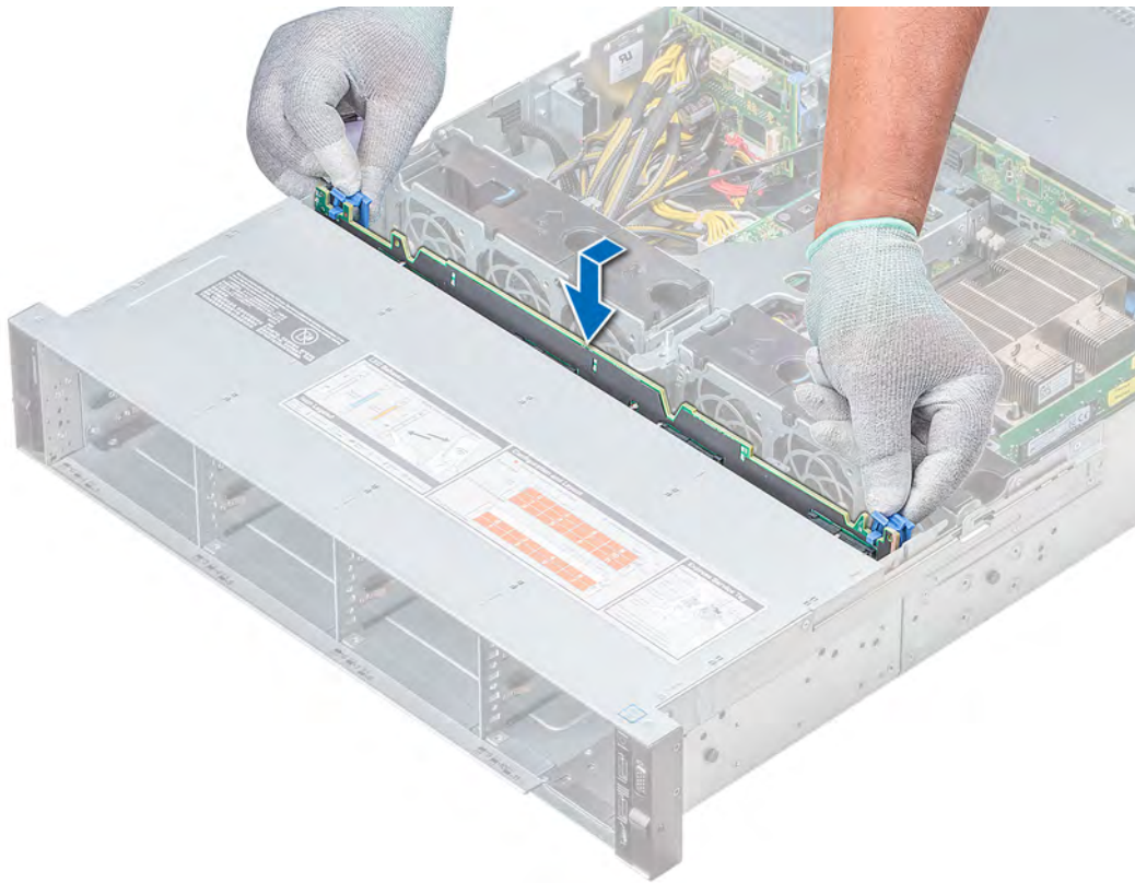
Figure 100. Installing the backplane
