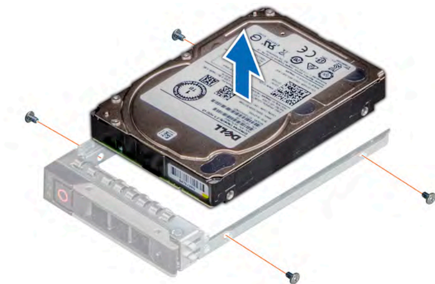
Figure 53. Removing the drive from the drive carrier
