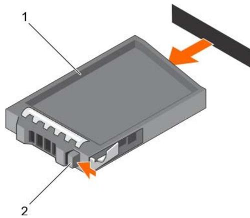
Figure 88. Removing a 2.5-inch hard drive blank
