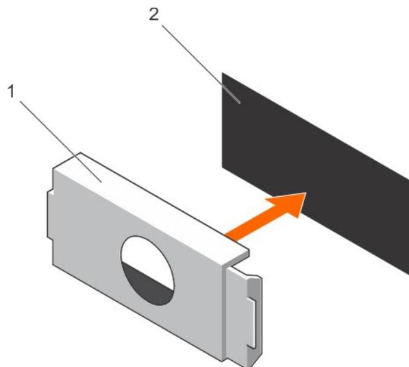
Figure 76. Installing the PSU blank
