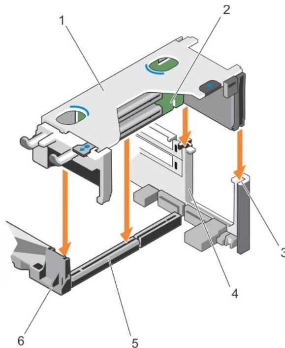
Figure 64. Installing the expansion card riser 1
