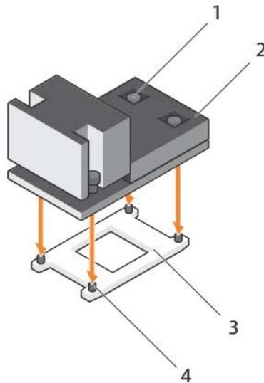
Figure 43. Installing the heat sink
