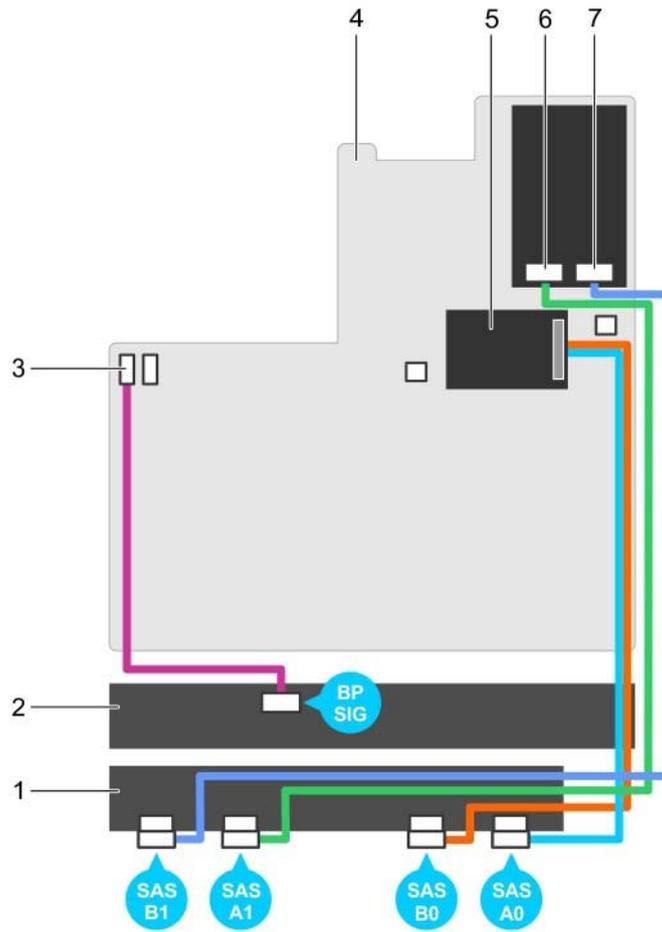
Figure 106. Cabling diagram—2.5 Inch (x24) SAS/SATA backplane (option 2)
