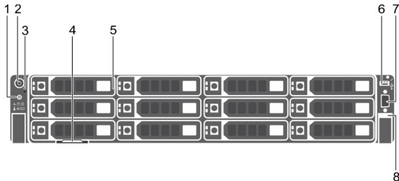
Figure 3. 12 x 3.5-inch hard drive chassis
