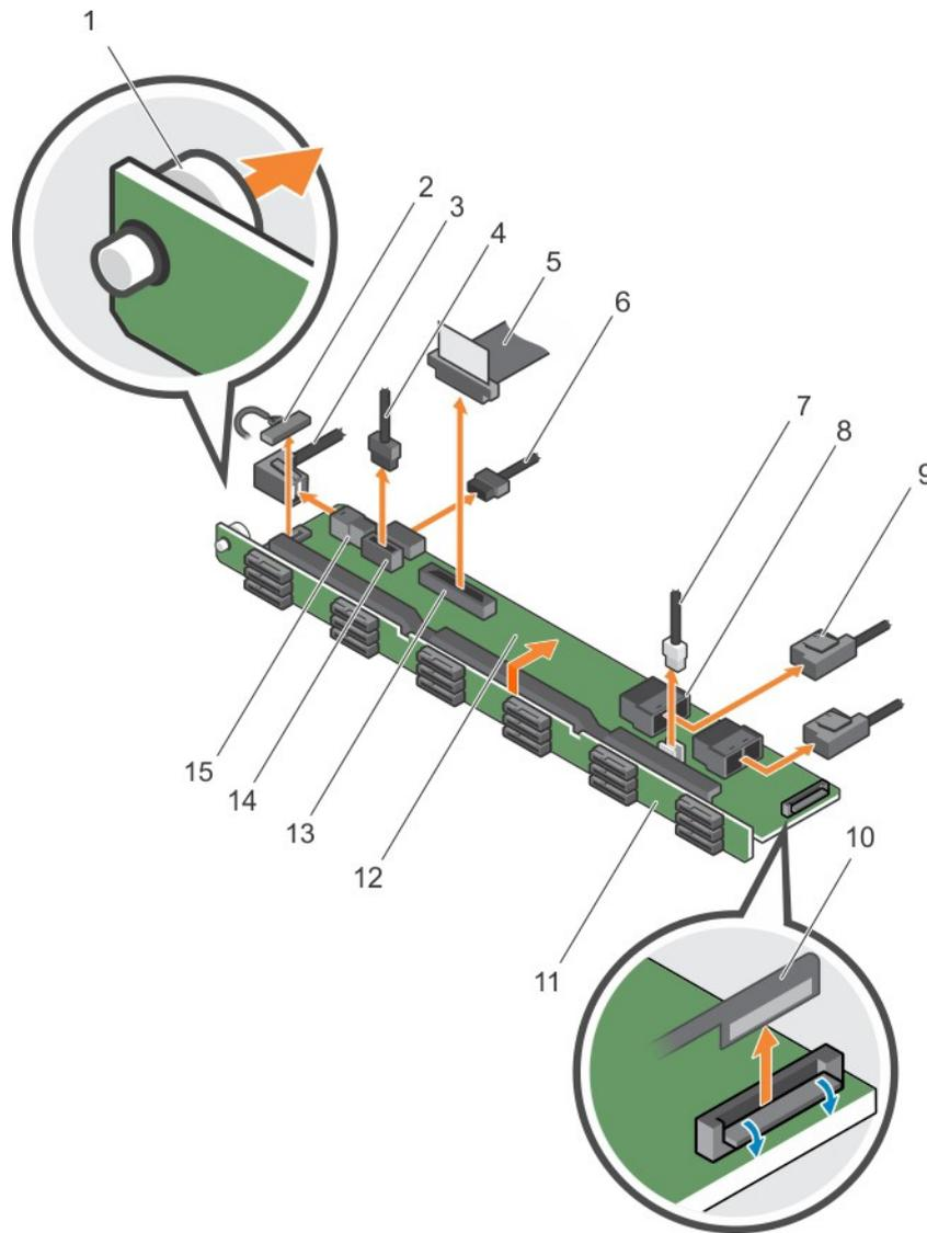
Figure 111. Removing the 1.8 Inch (x18) SAS/SATA backplane
