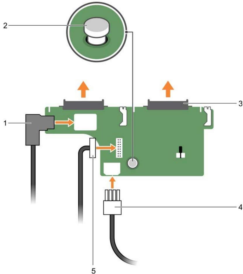
Figure 117. Installing the optional 2.5 inch (x2) hard drive backplane
