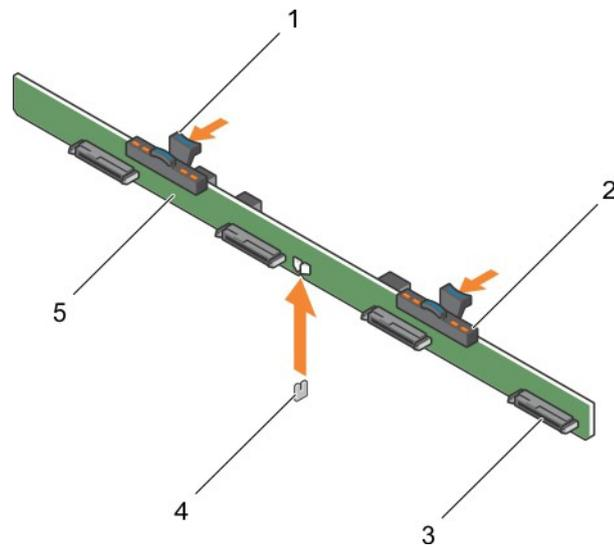
Figure 31. Removing the 3.5 inch (x4) hard drive backplane
