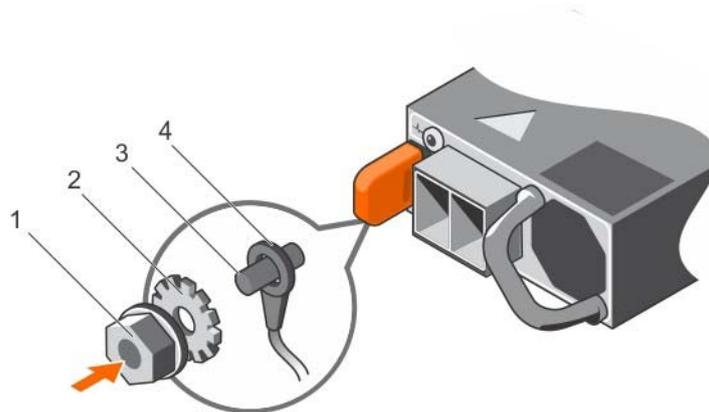
Figure 79. Assembling and connecting the safety ground wire
