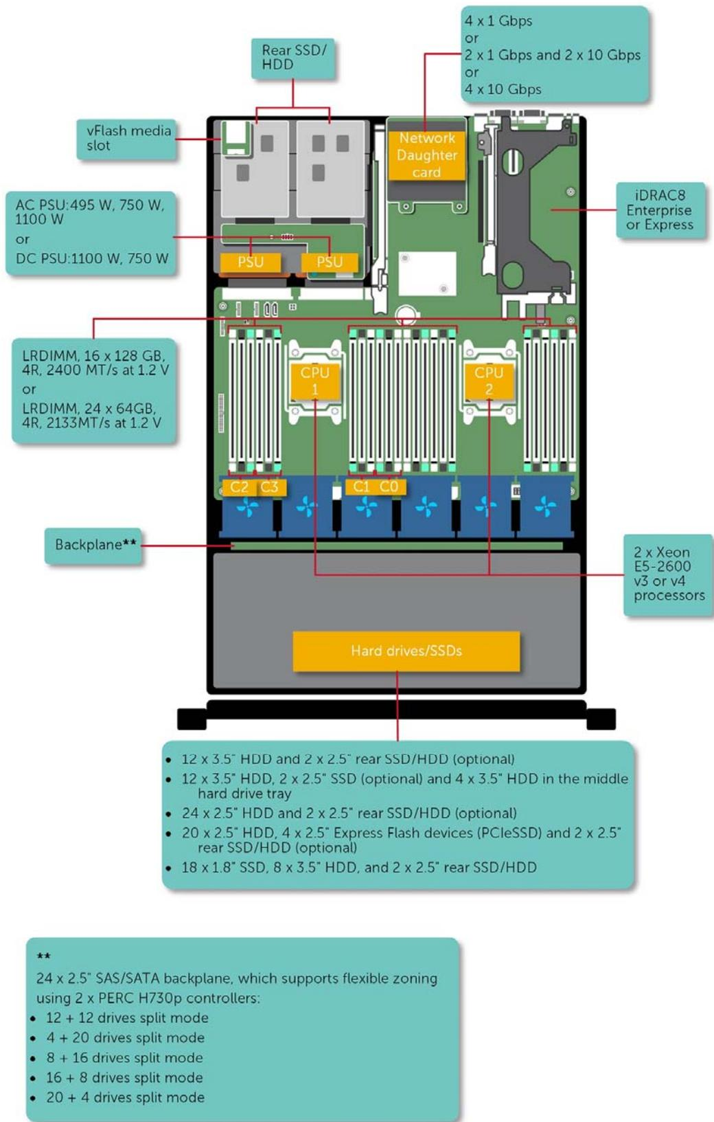
Figure 1. Supported configurations for the PowerEdge R730xd system
