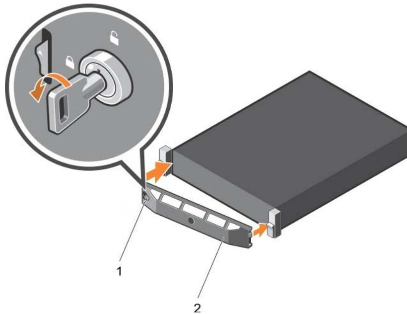
Figure 16. Installing the optional front bezel
