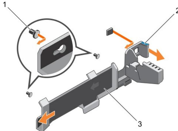
Figure 48. Removing the cable retention bracket
