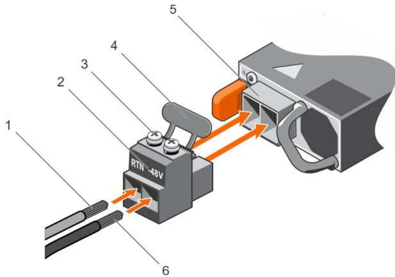
Figure 81. Assembling the DC Input Power Wires
