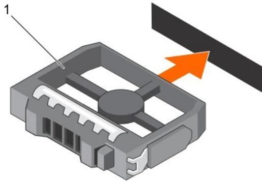
Figure 93. Installing a 3.5 inch hard drive blank
