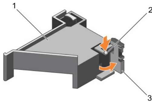
Figure 46. Opening the PCIe card holder latch
