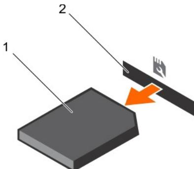
Figure 118. Removing the SD vFlash media card
