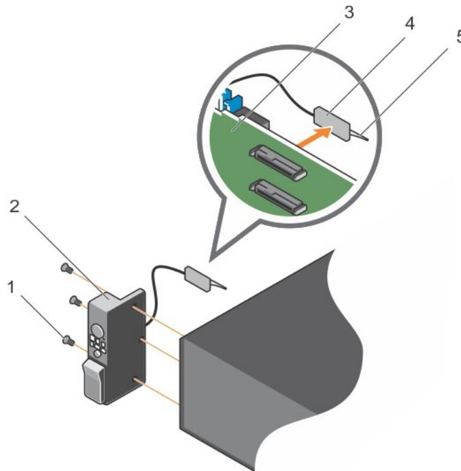
Figure 122. Removing the control panel
