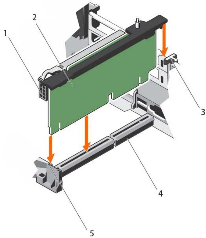
Figure 65. Installing the expansion card riser 2
