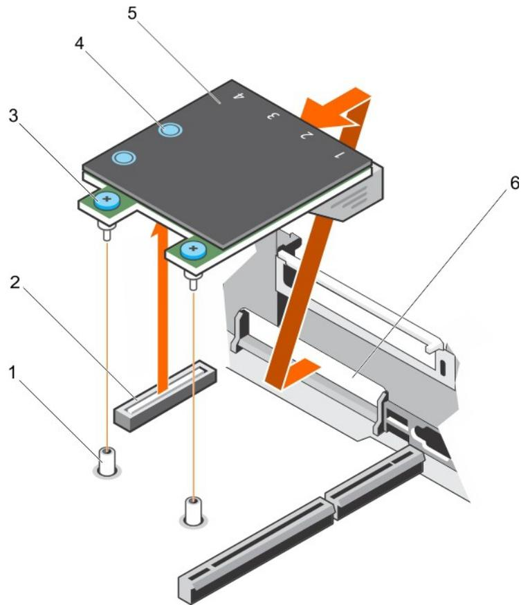
Figure 69. Removing the NDC
