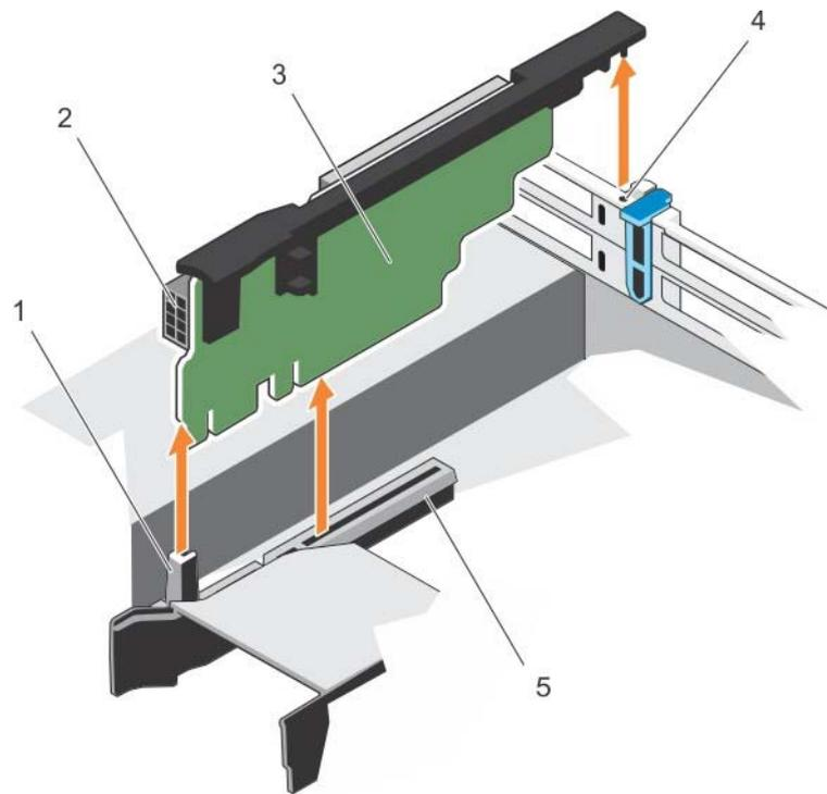
Figure 62. Removing the expansion card riser 3
