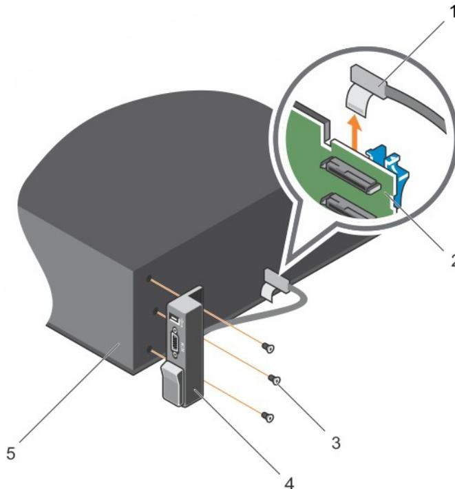
Figure 124. Removing the I/O panel
