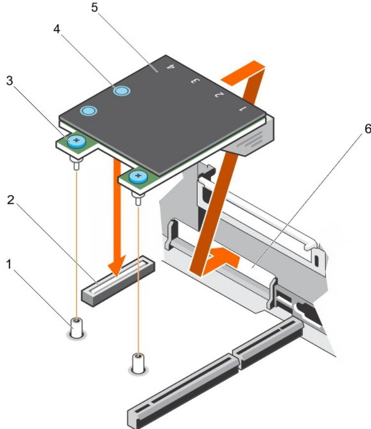
Figure 70. Installing the NDC
