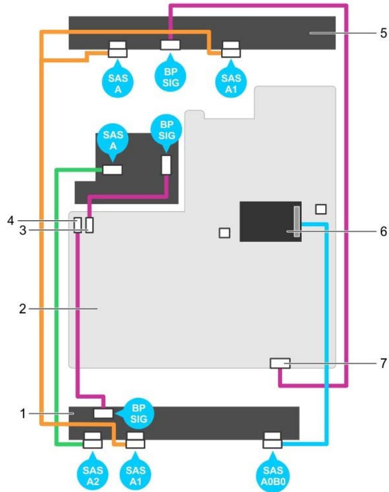
Figure 110. Cabling diagram—3.5 inch (x12) SAS/SATA backplane (option 2)
