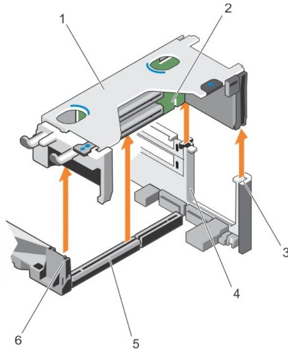
Figure 58. Removing the expansion card riser 1
