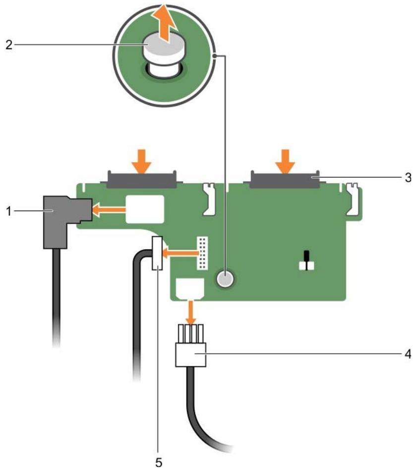
Figure 116. Removing the optional 2.5 inch (x2) hard drive backplane
