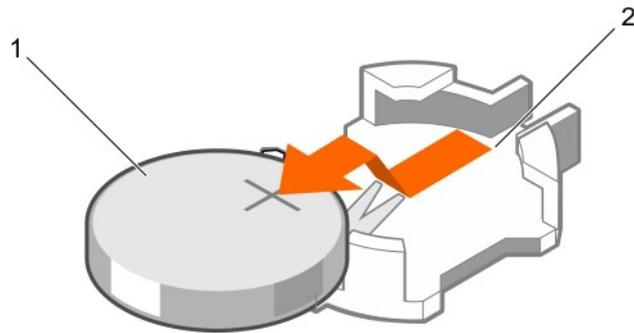
Figure 73. Removing the system battery
