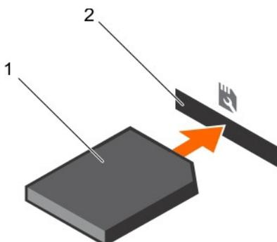
Figure 119. Installing the SD vFlash media card
