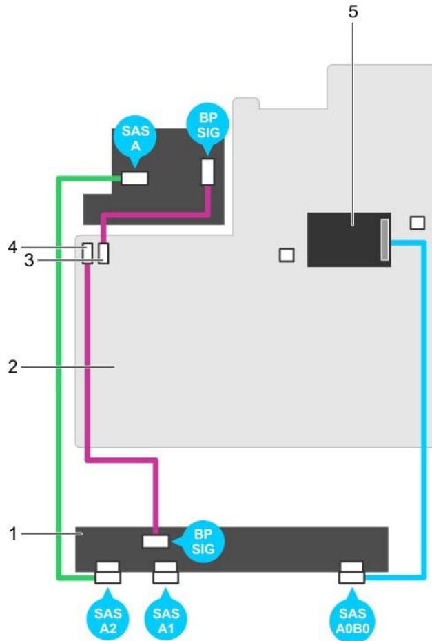
Figure 109. Cabling diagram—3.5 inch (x12) SAS/SATA backplane (option 1)
