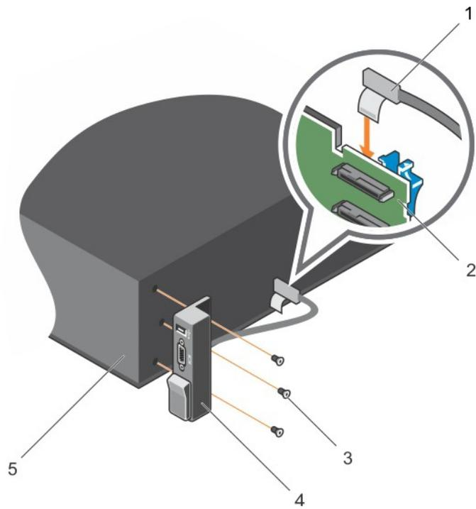
Figure 125. Installing the I/O panel
