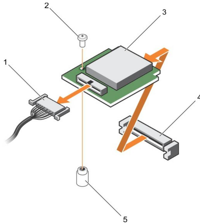
Figure 120. Removing the vFlash media unit
