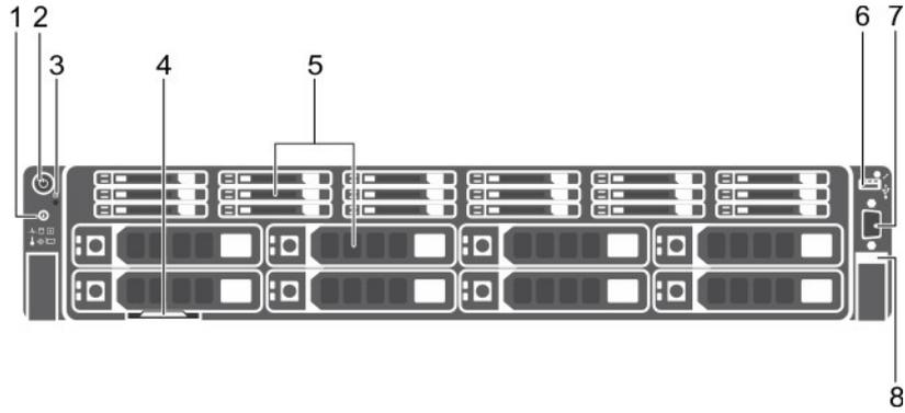
Figure 4. 8 x 3.5-inch hard drive and 18 x 1.8-inch SSD chassis
