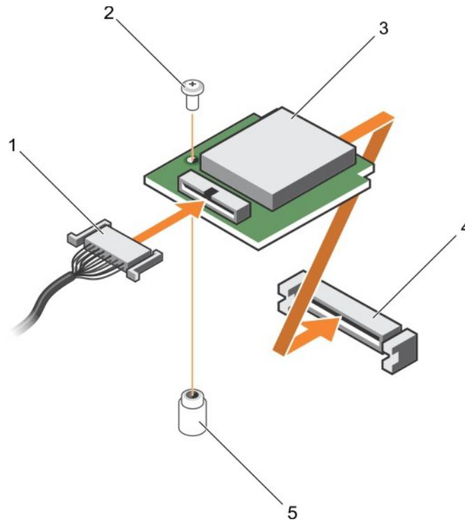
Figure 121. Installing the vFlash media unit
