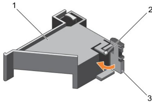
Figure 47. Closing the PCIe card holder latch
