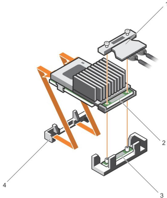
Figure 50. Removing the integrated storage controller card
