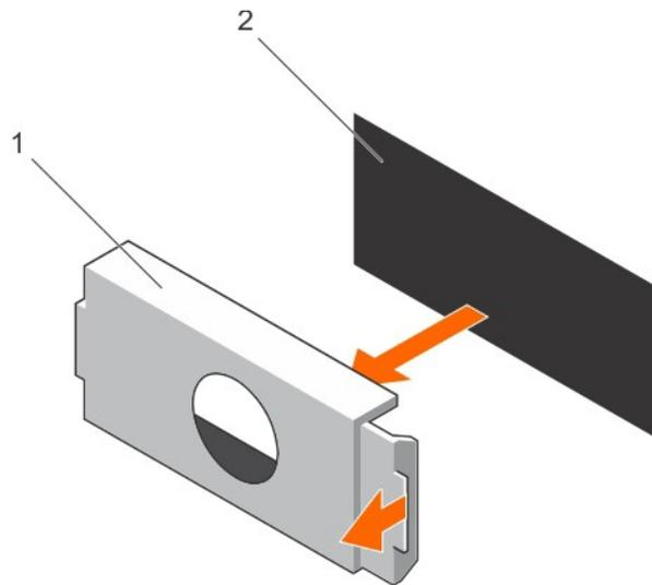
Figure 75. Removing the PSU blank
