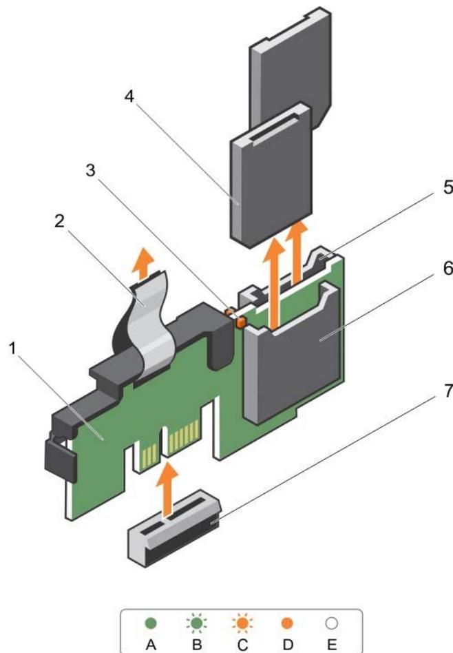
Figure 67. Removing the internal dual SD module (IDSDM)
