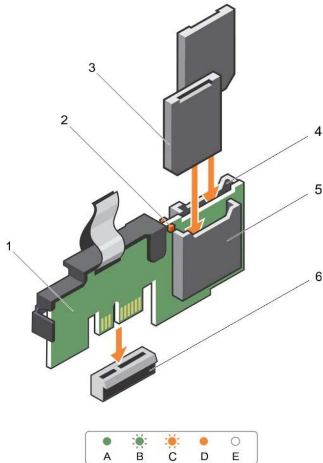
Figure 68. Installing the optional internal dual SD module
