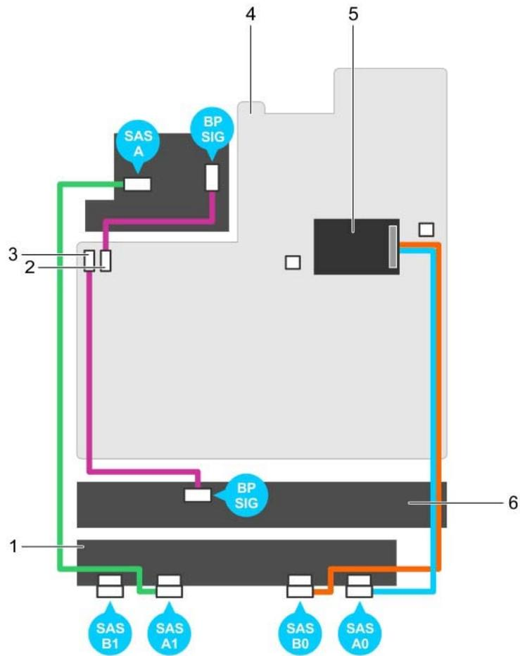
Figure 105. Cabling diagram—2.5 Inch (x24) SAS/SATA backplane (option 1)
