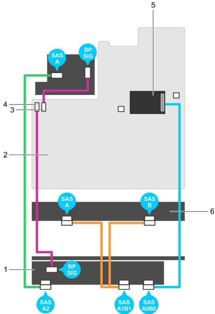
Figure 112. Cabling diagram—1.8 Inch (x18) SAS/SATA backplane
