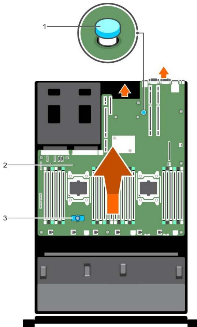
Figure 86. Installing the system board
