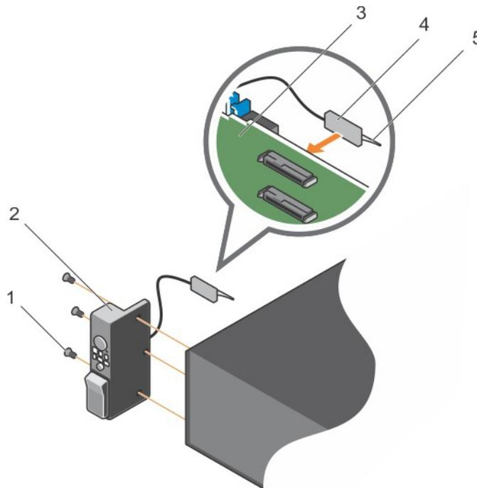
Figure 123. Installing the control panel
