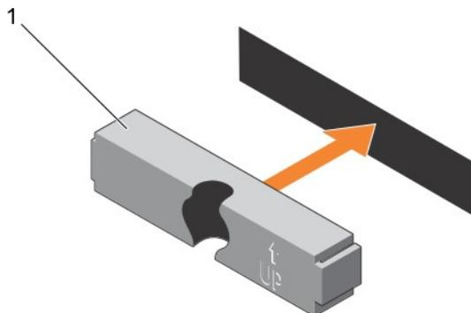
Figure 91. Installing a 2.5 inch hard drive blank (rear)
