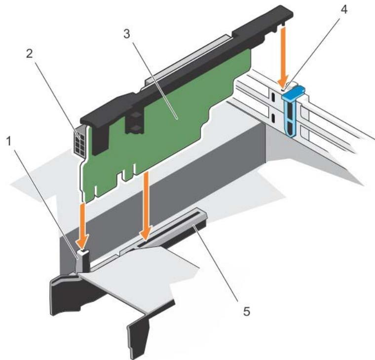
Figure 66. Installing the expansion card riser 3
