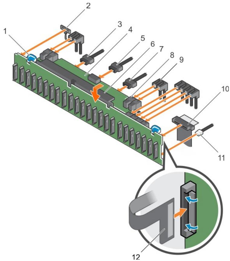
Figure 113. Installing the 2.5 inch (x24) SAS/SATA backplane
