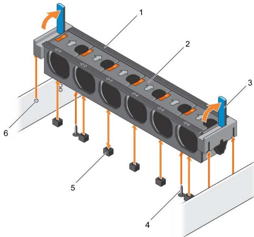
Figure 34. Removing the cooling fan assembly
