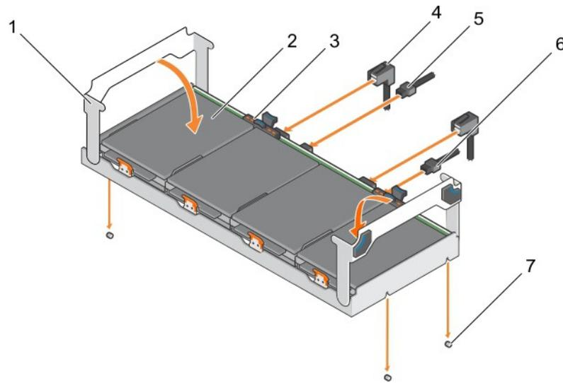
Figure 24. Installing the hard drive tray
