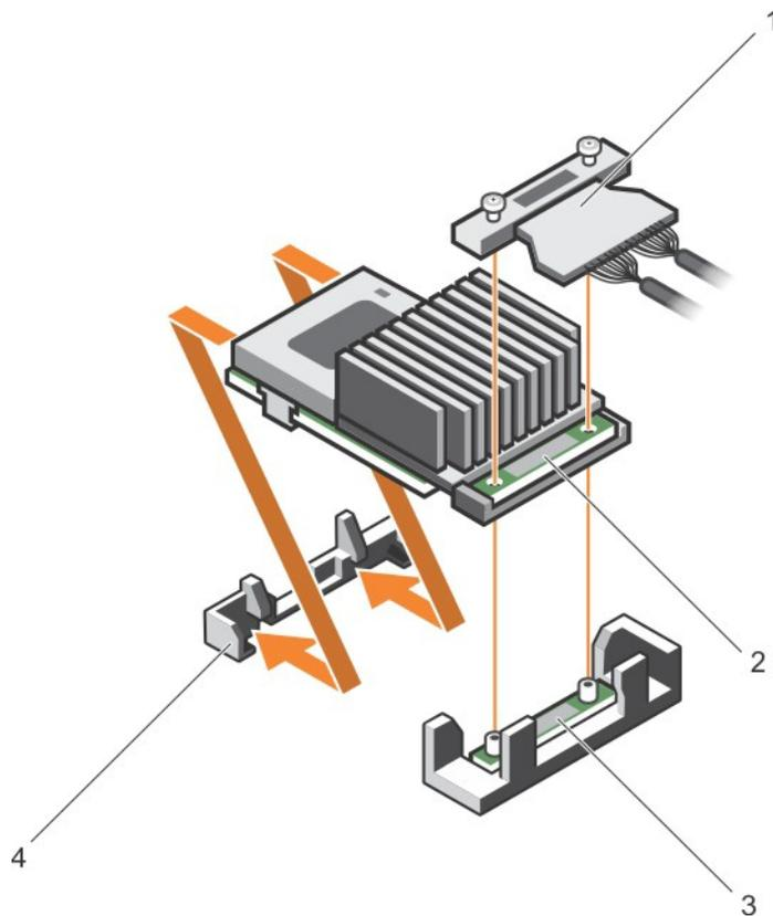
Figure 51. Installing the integrated storage controller card
