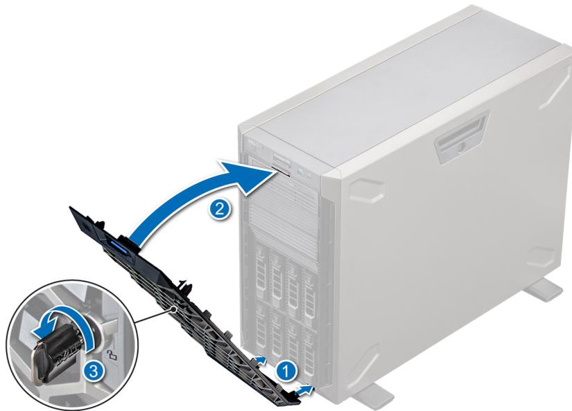
Figure 18. Installing the front bezel
