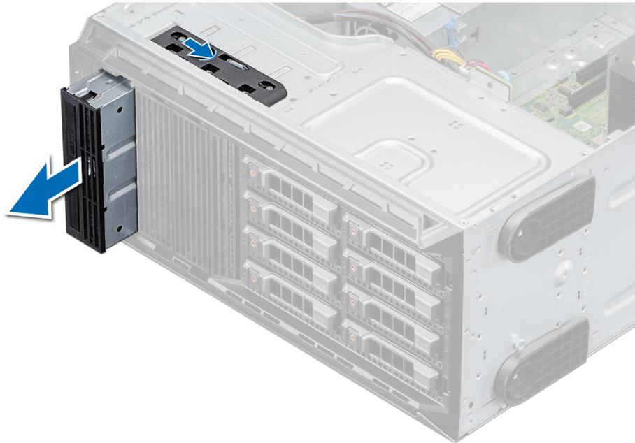
**Figure 40. Removing the optical drive**
