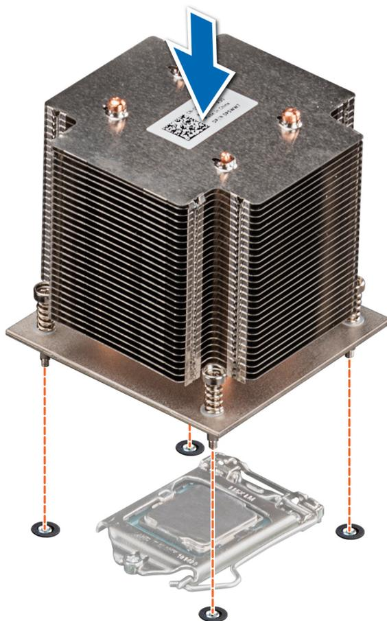
Figure 69. Installing the heat sink
