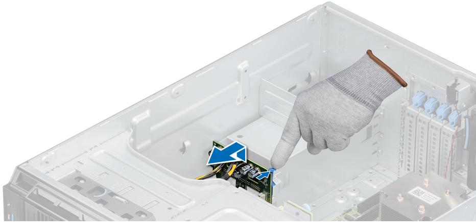
**Figure 76. Removing the power interposer board**
