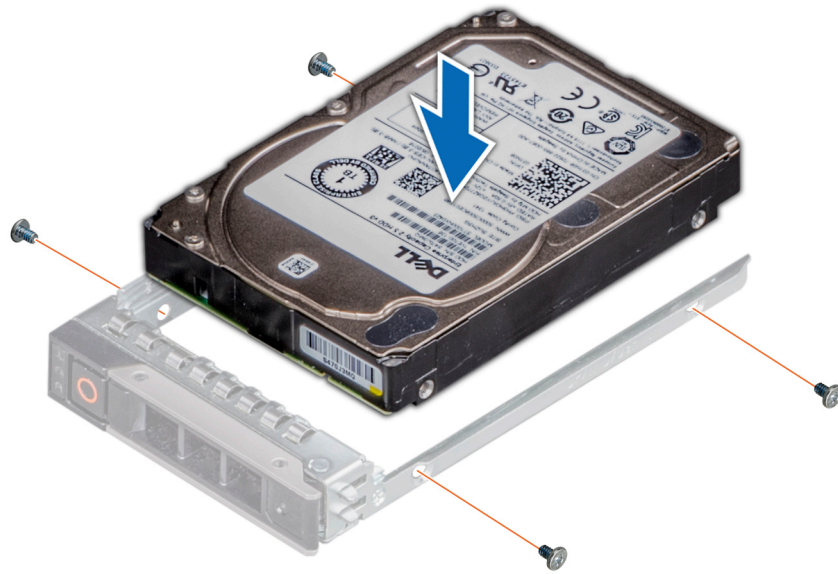
Figure 45. Installing a drive into the drive carrier
