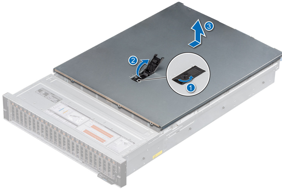
Figure 20. Removing the system cover
