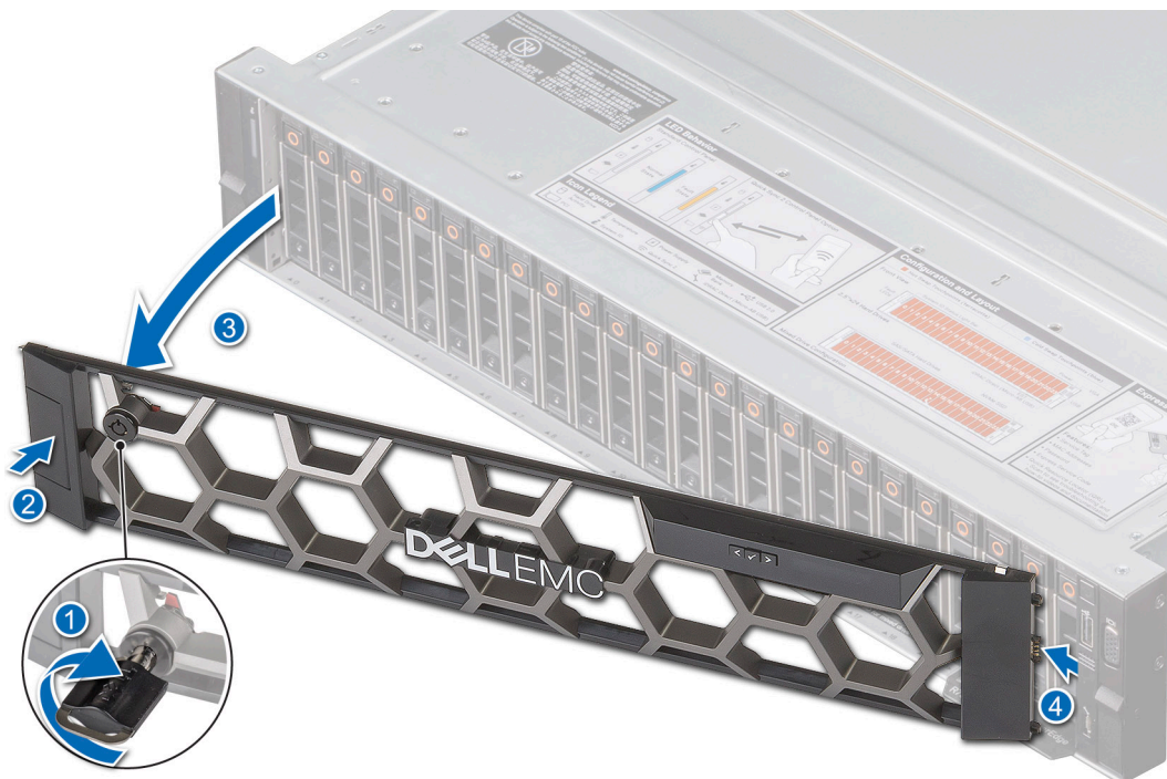
Figure 18. Removing the front bezel
