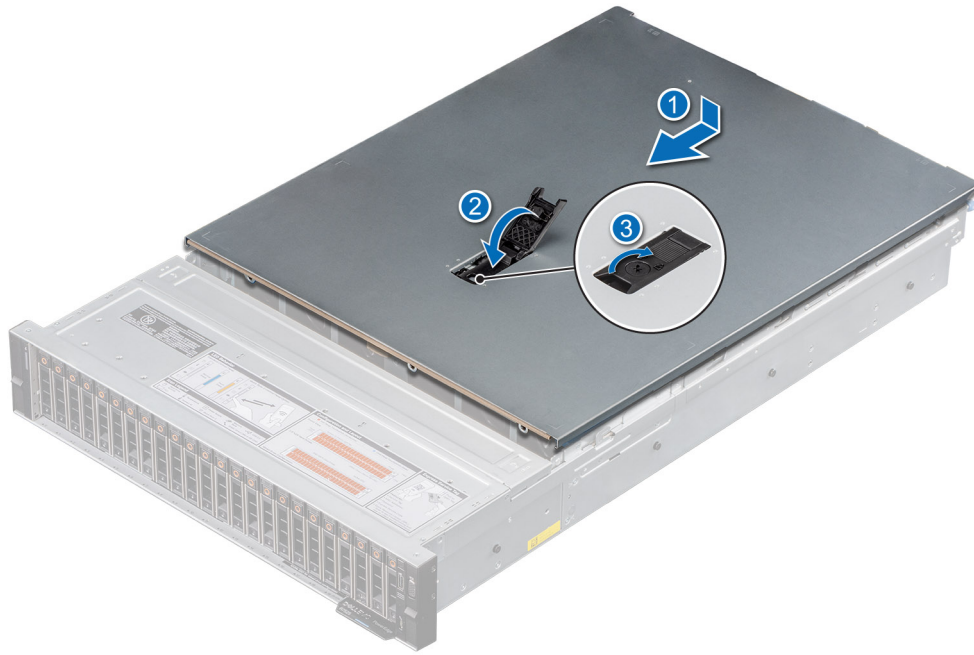
Figure 21. Installing the system cover
