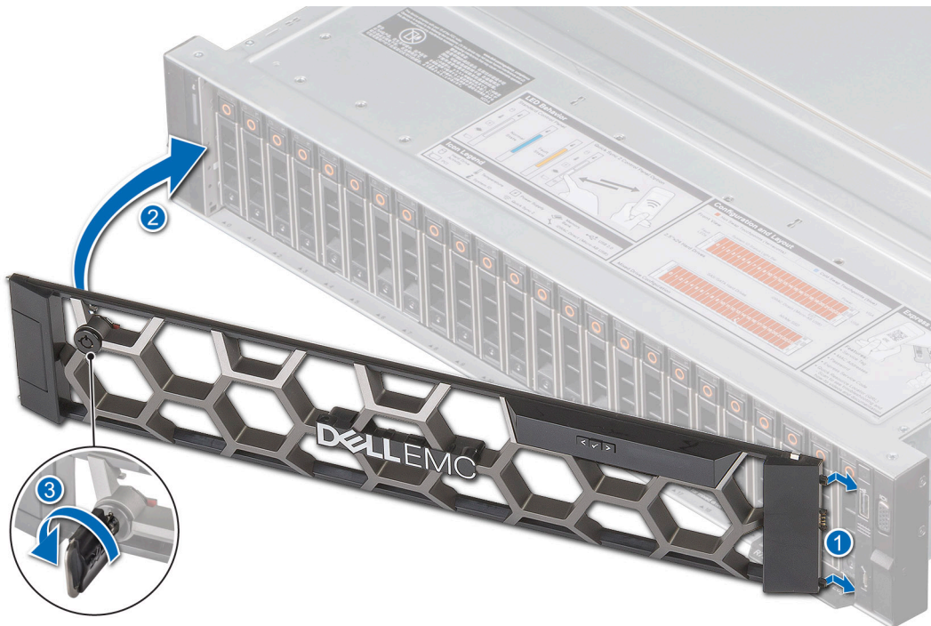
Figure 19. Installing the front bezel
