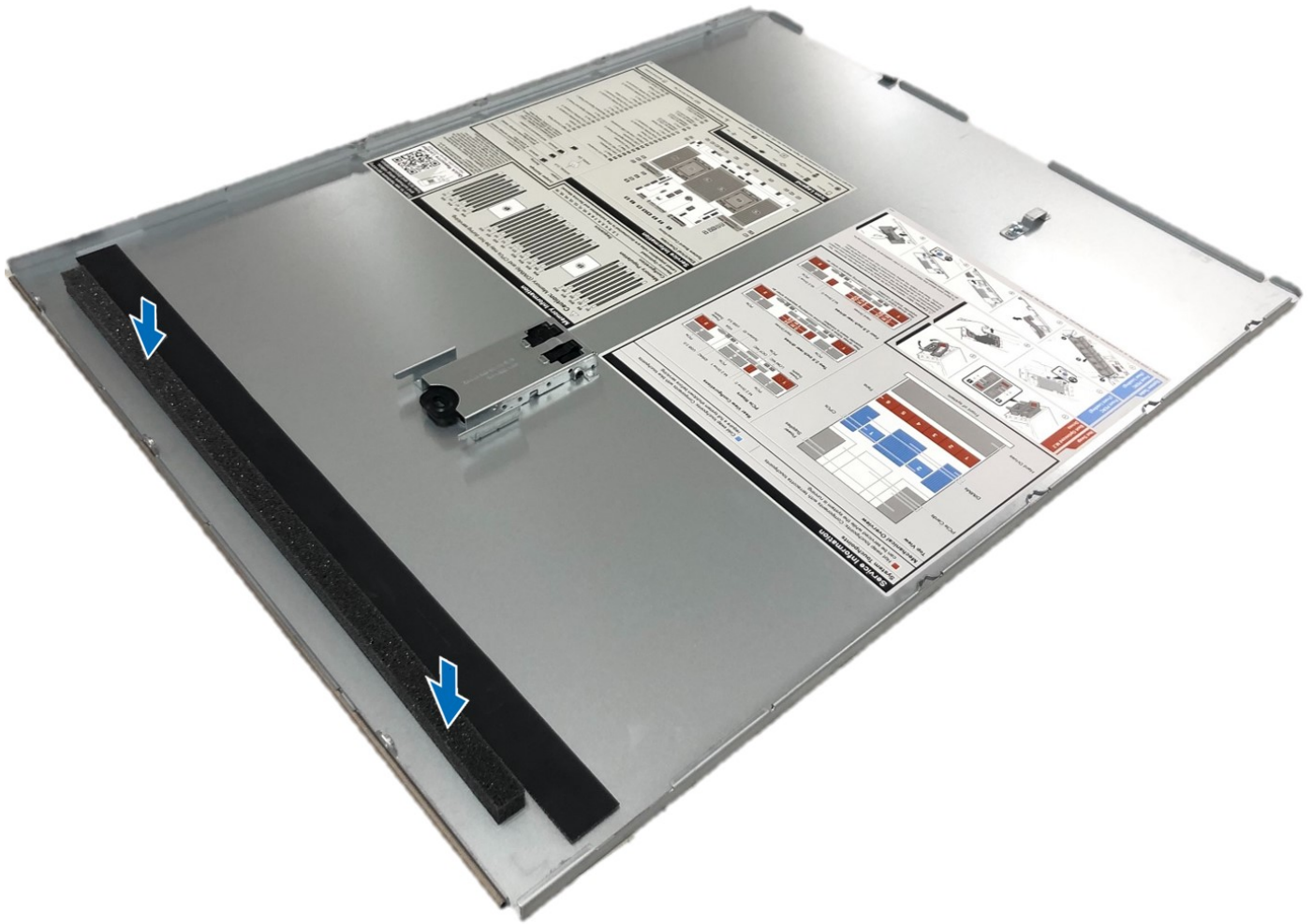
Figure 155. Installing Mylar foam on the system cover
