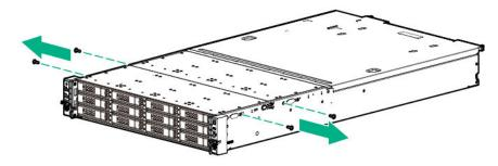
Keep the shipping screws and the system packaging materials in case there is a need to ship or transport the system at a later date.
