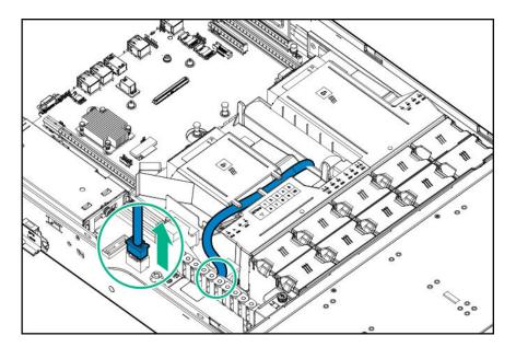
8. Remove the cable from the air baffl clips, then remove the HPE Smart Storage Battery from the air baffle
