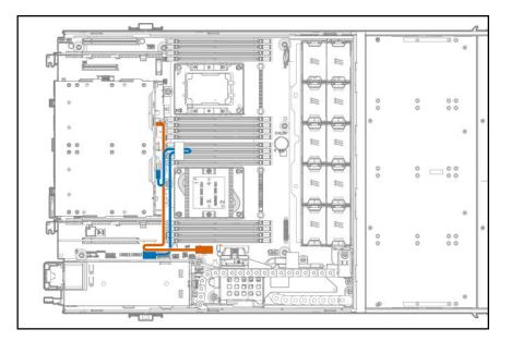
• Rear LFF drive cage connected to PCIe card in slot 1 or 2
