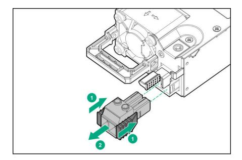
**5.** Loosen the screws on the terminal block connector.
