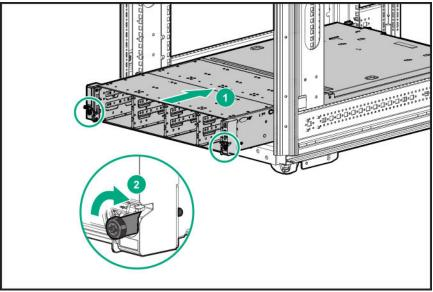
5. Make sure the pins on the chassis retention brackets slot into the notches located on both sides of the chassis.
