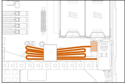
• Internal drive cage P3 connected to rear LFF drive cage
