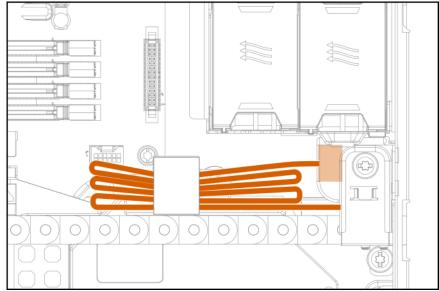
• Internal drive cage P1 and P2 connected to P1 and P2 on a PCIe card in slot 5
