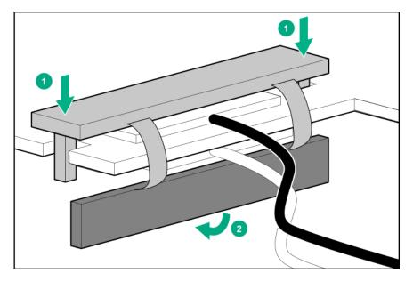
**d.** Connect the other end of the black and white cables to the auxiliary card. Be sure that the cables on both cards are angled in the same direction after installation.
