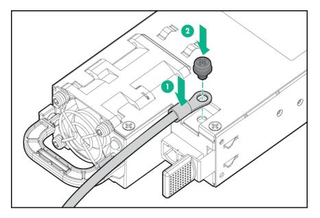
7. Insert the -48 V wire into the left side of the terminal block connector, and then tighten the screw to 1.3 N m (10 lb-in) of torque.
