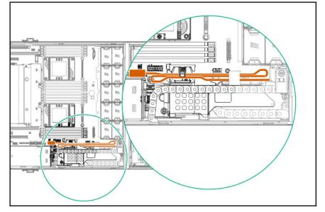
• Unused internal drive cage P2 cable folded and stored in the wider slot of the cable guard
