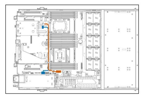
• Rear SFF drive cage connected to PCIe card in riser slot 4
