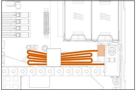
• Internal drive cage P1 and P2 connected to P1 and P2 on a PCIe card located in slot 3 or 4 in riser
