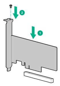
• Installing the adapter in slot 3 in the riser cage
