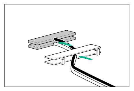
**b.** The white and black cables from the auxiliary card connect to the adapter board ports labeled WHITE CABLE and BLACK CABLE, respectively. The cable latch door must be open when connecting the cables. Close the cable latch door after connecting the cable.
