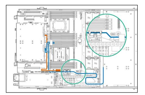
• Internal drive cage P3 connected to the rear SFF drive cage
