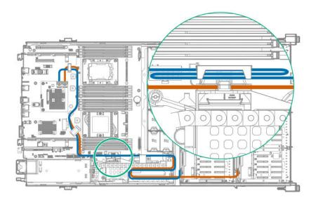
• Unused front drive cage P2 cable folded and stored in the narrow slot of the cable guard
