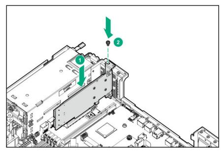
• M.2 SSD enablement board installed in the onboard PCIe3 x16 expansion slot 1
