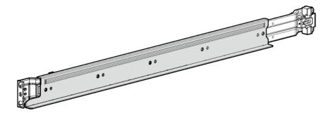
Install the chassis retention brackets on the non-shelf portion of the rack rail.
