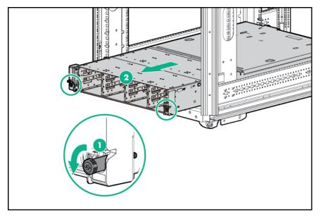
c. Press the system release latches, and then slide the system out of the rack.
