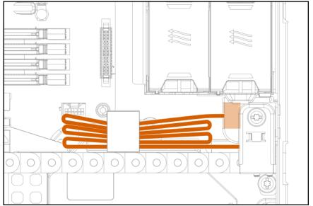
• Internal drive cage P1 and P2 connected to P1 and P2 on a PCIe card in slot 1
