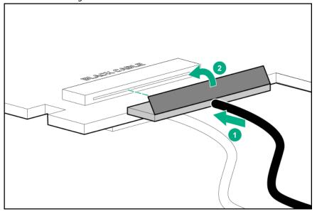
c. Slide the cable retention clip up and connect it to the adapter board over the cable connectors.
