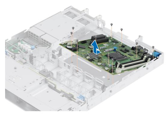
Figure 77. Removing the system board
