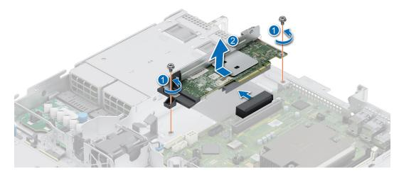
Figure 63. Removing the PERC card
