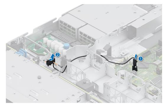
Figure 17. Removing the intrusion switch module
