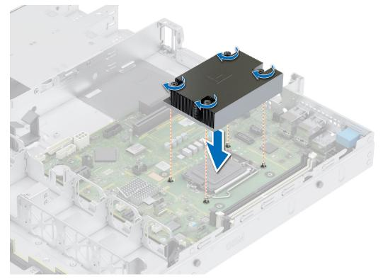
Figure 42. Installing the heat sink
