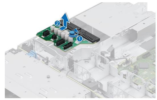
Figure 71. Removing the power interposer board
