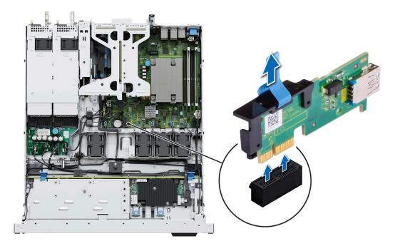
Figure 65. Removing the internal USB card
