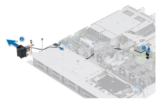
Figure 80. Removing the left control panel
