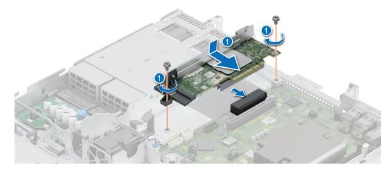
Figure 64. Installing the PERC card
