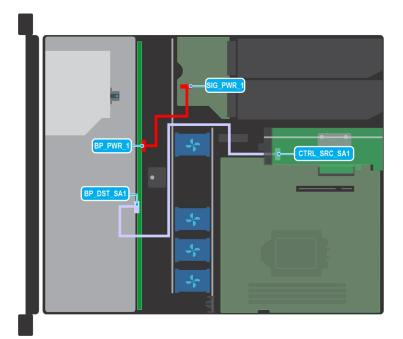
Figure 23. Cable routing - 4 x 3.5-inch drive SAS or SATA backplane
