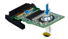
Figure 79. Installing the TPM
