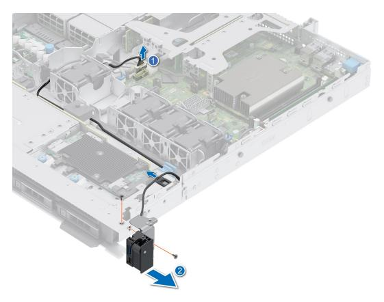
Figure 82. Removing the right control panel
