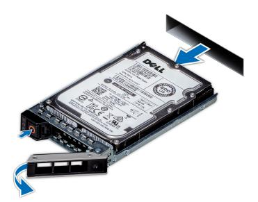
Figure 29. Removing a drive carrier
