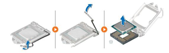
Figure 43. Removing the processor
