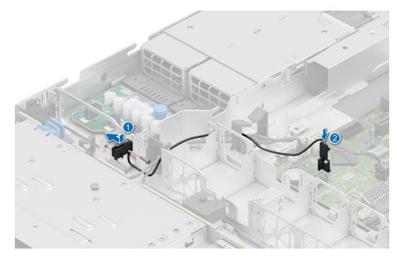
Figure 18. Installing the intrusion switch
