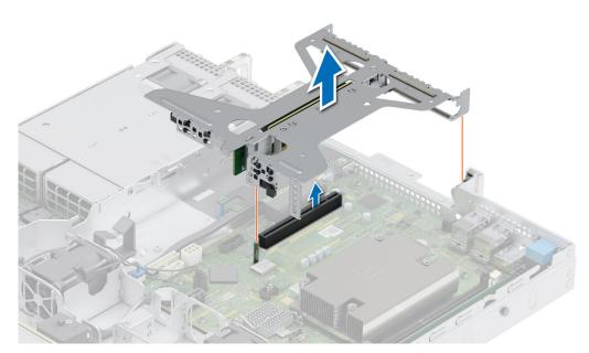
Figure 47. Removing the butterfly riser
