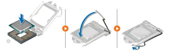
Figure 44. Installing the processor
