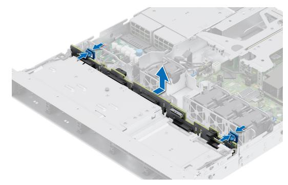
Figure 21. Removing the backplane
