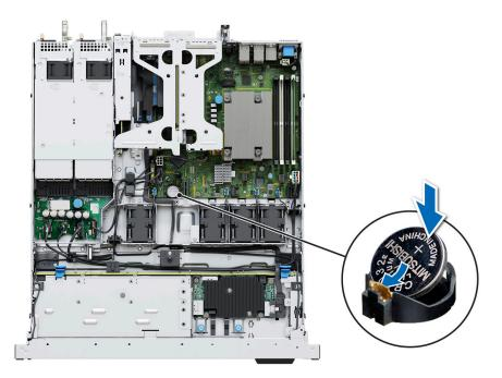
Figure 60. Installing the system battery
