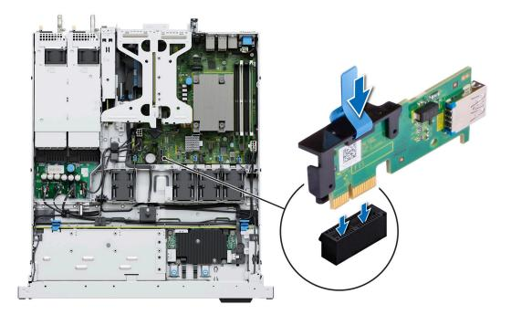
Figure 66. Installing the internal USB card
