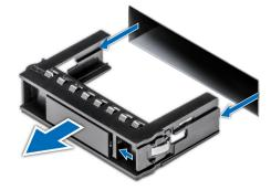
Figure 33. Removing a drive blank
