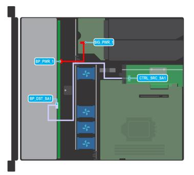
Figure 26. Cable routing - 8 x 2.5-inch drive SATA backplane with internal PERC
