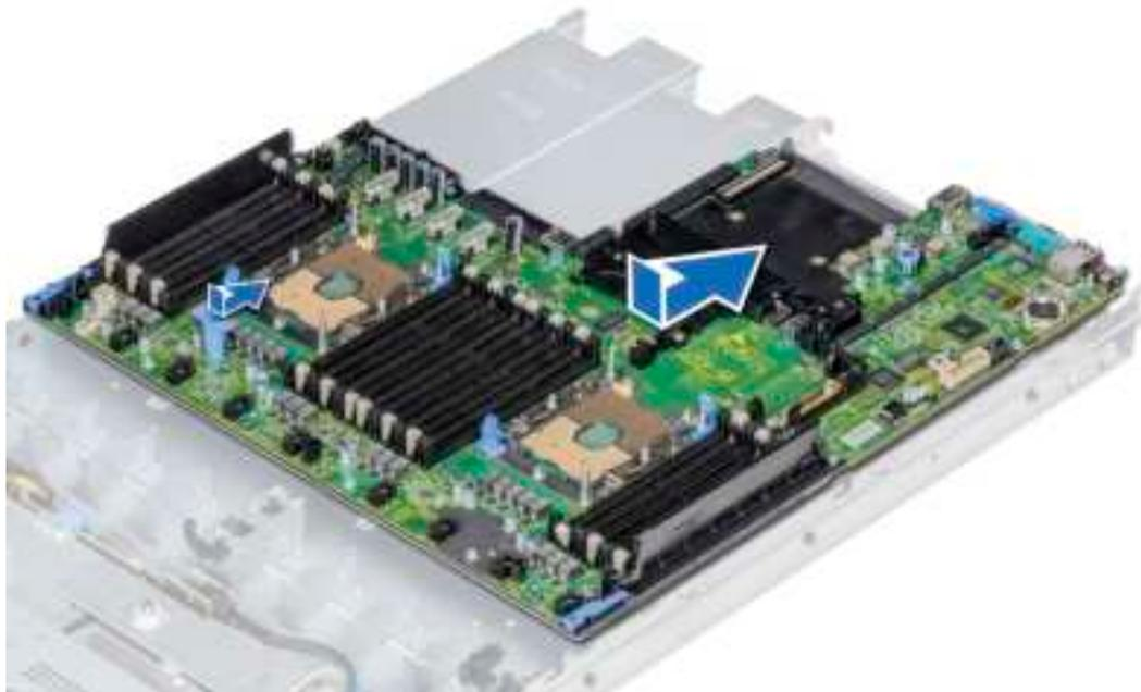
**Figure 110. Installing the system board**
