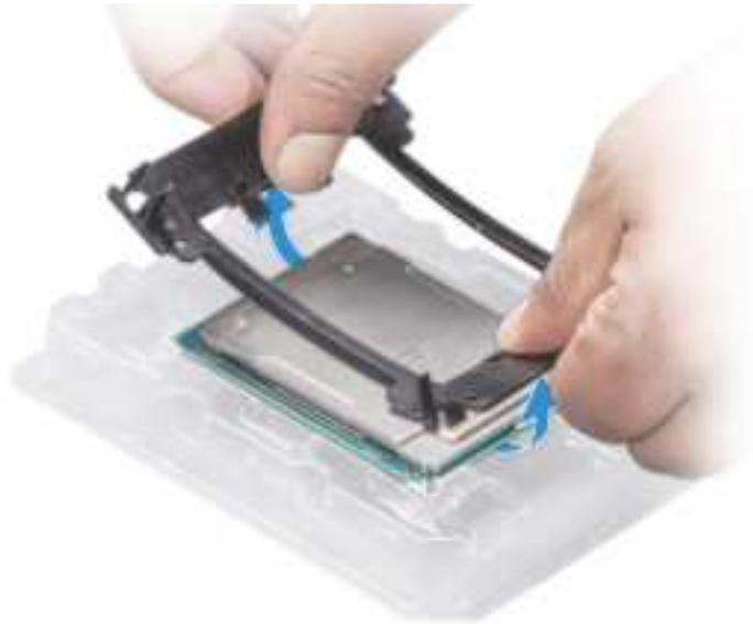
**Figure 45. Removing the processor bracket**
