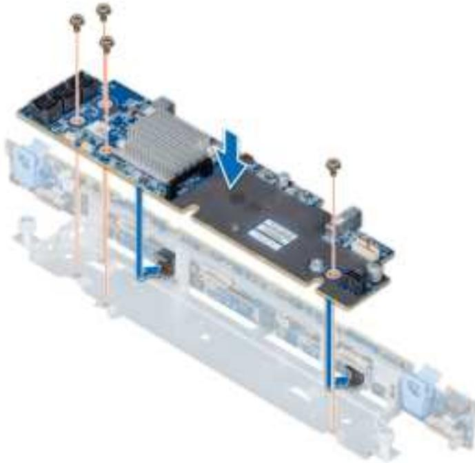
**Figure 94. Installing the SAS expander card**
