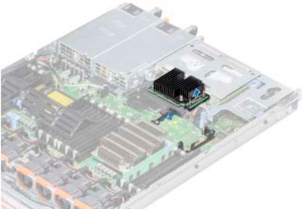
**Figure 76. Removing the integrated storage controller card**
