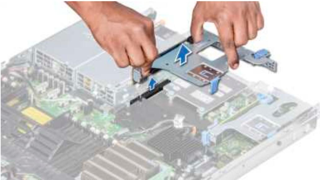
**Figure 53. Removing the expansion riser 2B**
