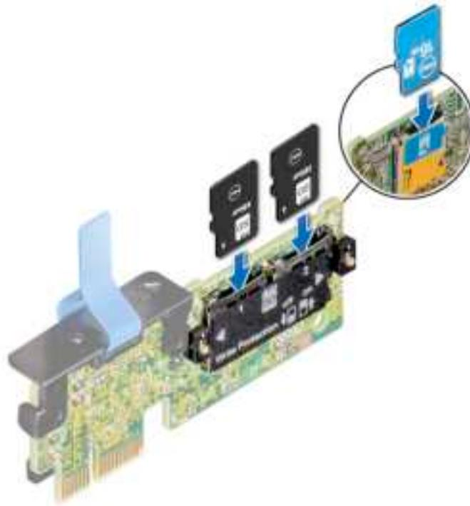
**Figure 72. Installing the MicroSD card**
