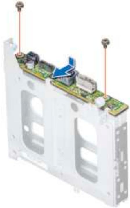
**Figure 86. Installing the 2.5 inch drive rear backplane**
