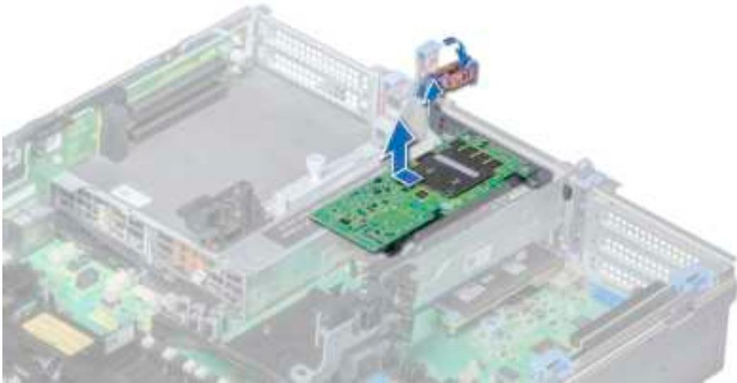
Figure 60. Removing the expansion card from expansion card riser 2
