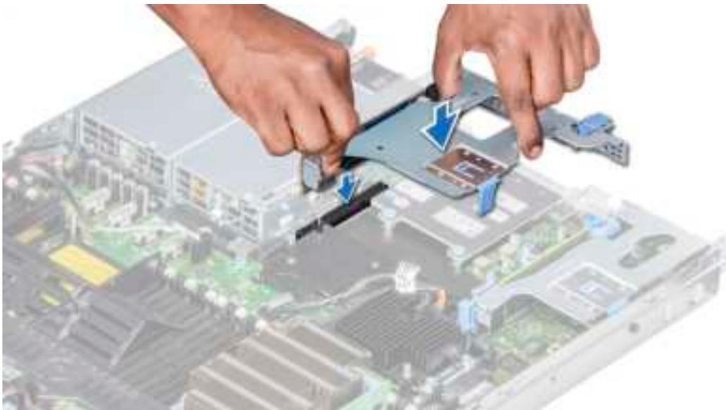
**Figure 57. Installing the expansion riser 2B**
