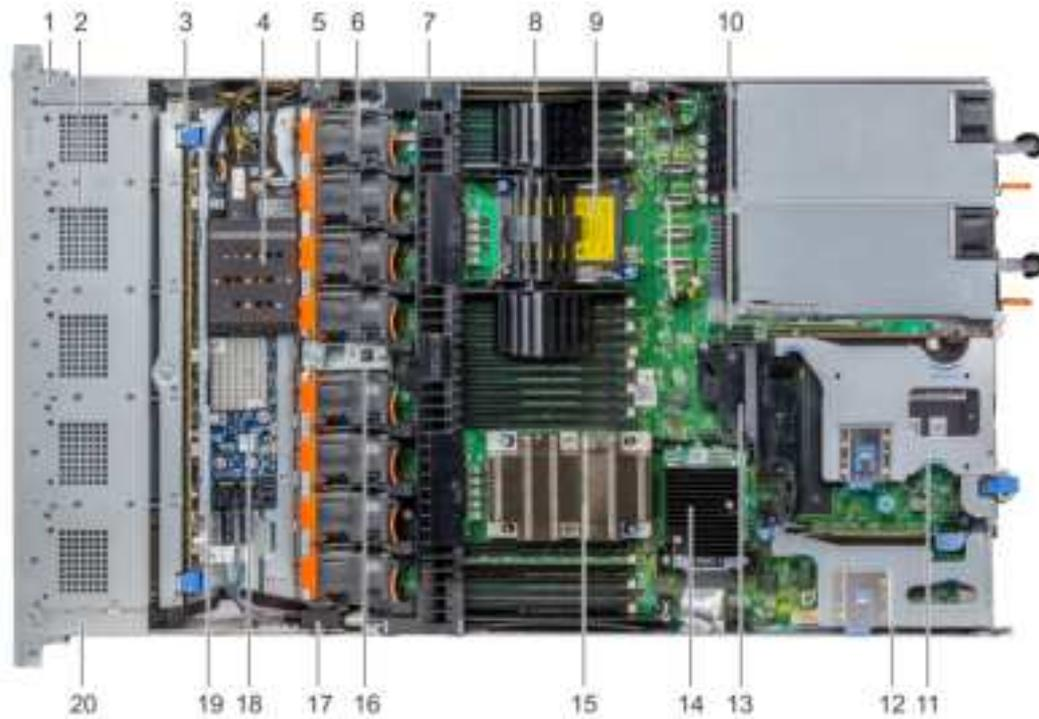
**Figure 32. Inside the system - 2 PCIe expansion risers**
