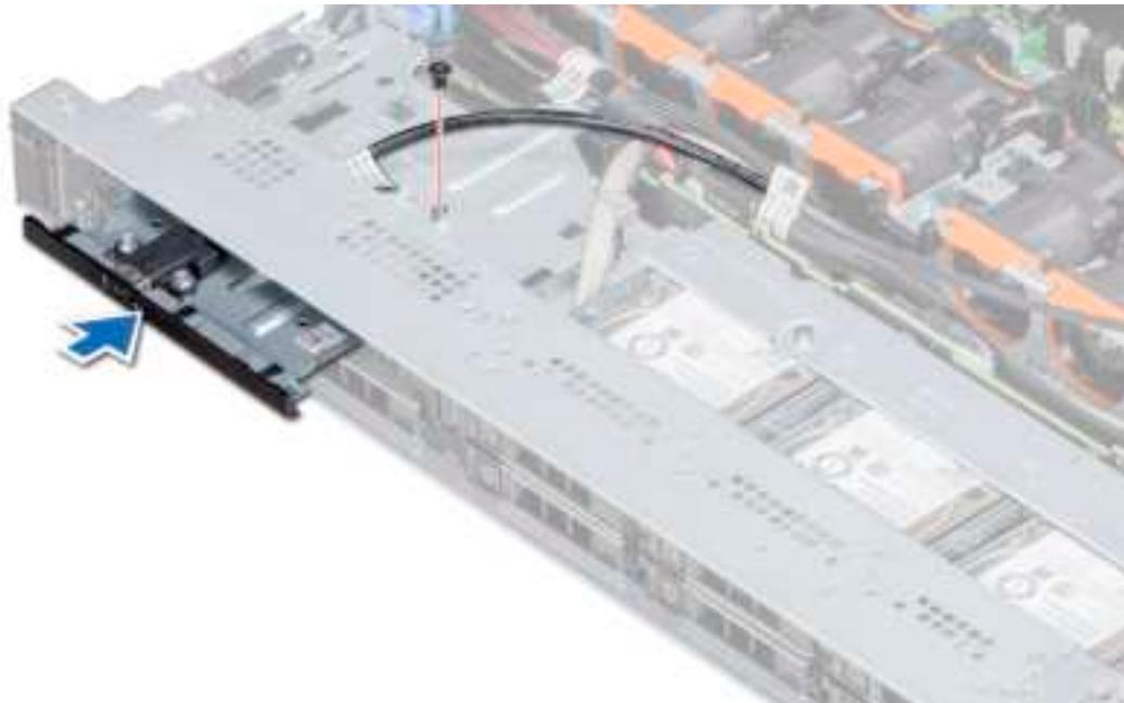
Figure 100. Installing the USB module
