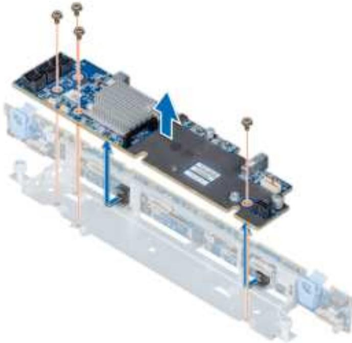
**Figure 93. Removing the SAS expander card**
