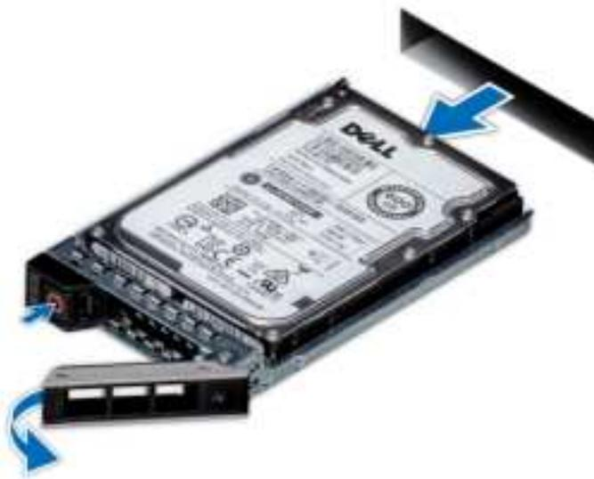
Figure 25. Removing a drive carrier
