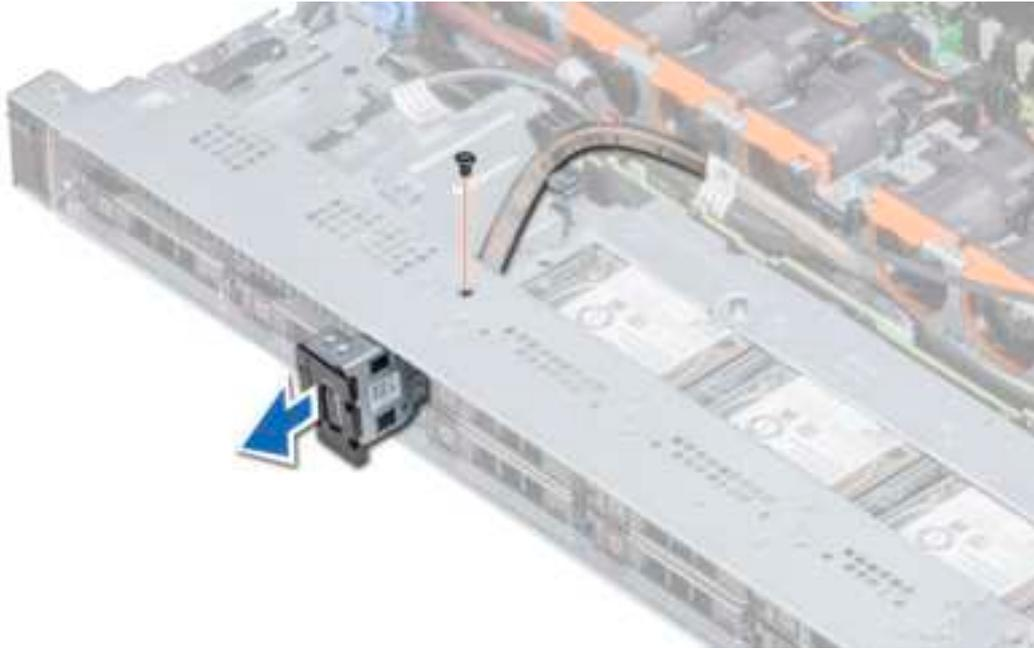
**Figure 101. Removing the VGA module**
