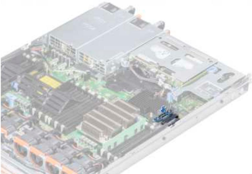
**Figure 78. Installing the integrated storage controller card cable**
