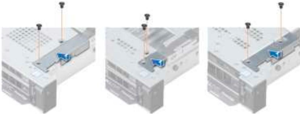
**Figure 119. Installing the cable cover**
