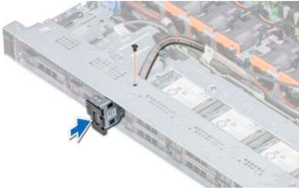
**Figure 102. Installing the VGA module**
