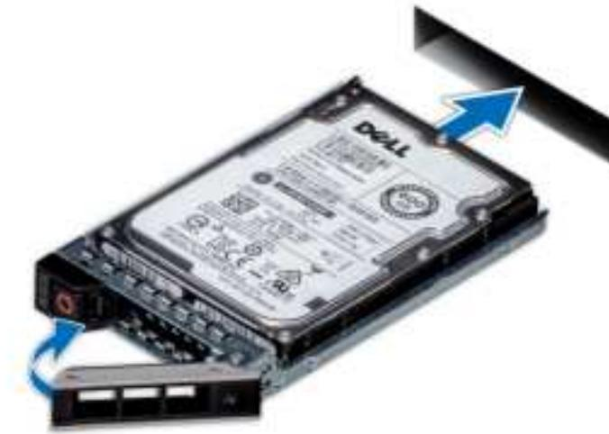
**Figure 26. Installing a drive carrier**
