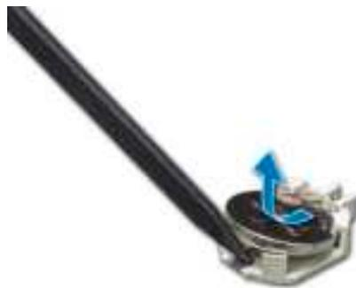
**Figure 97. Removing the system battery**
