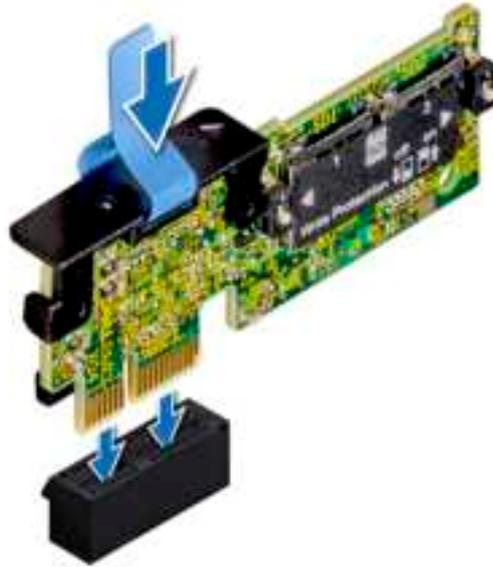
**Figure 70. Installing optional IDSDM module**
