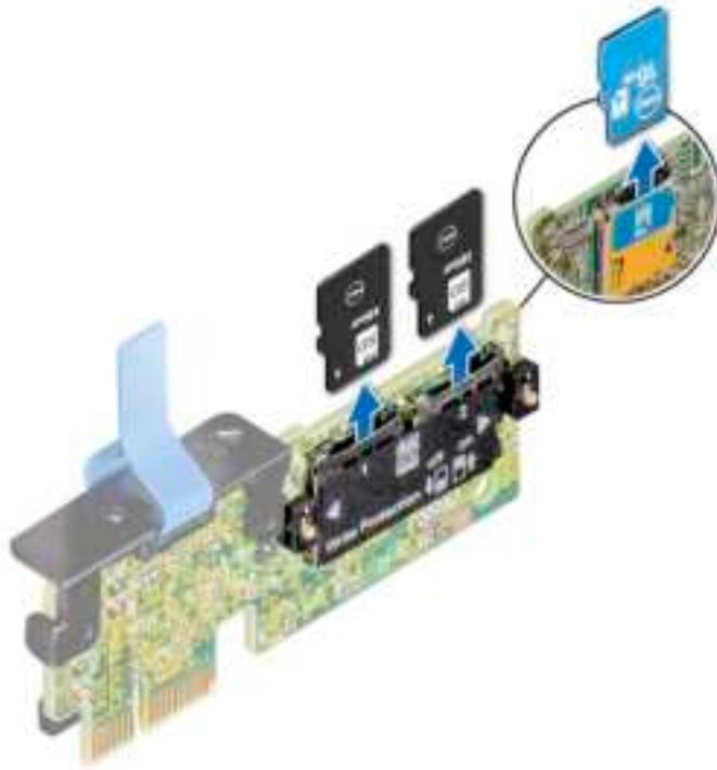
**Figure 71. Removing the MicroSD card**
