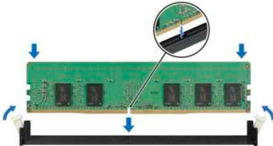
Figure 40. Installing a memory module
