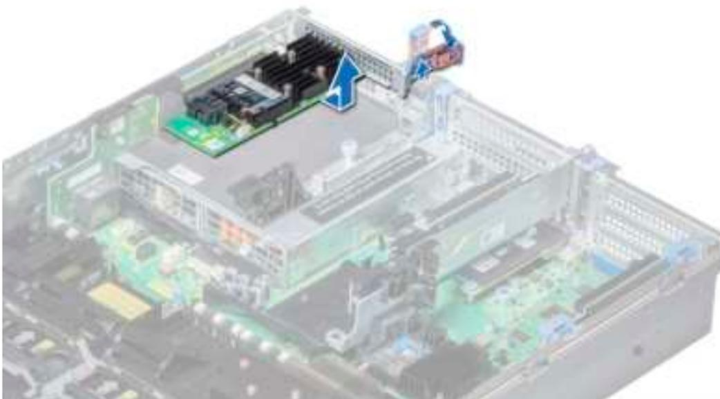
Figure 61. Removing the expansion card from expansion card riser 3
