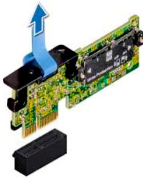
**Figure 69. Removing the optional IDSDM module**
