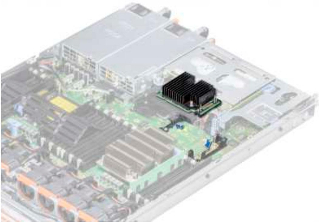
**Figure 77. Installing the integrated storage controller card**
