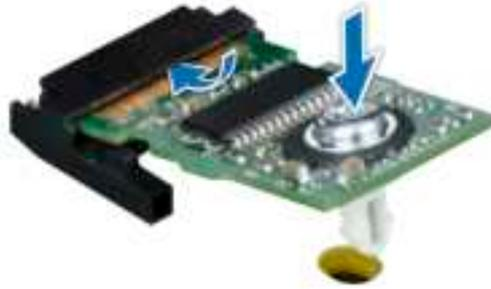
Figure 111. Installing the TPM
