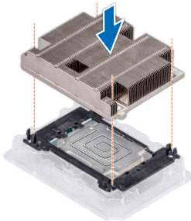
**Figure 48. Installing the heat sink onto the processor**
