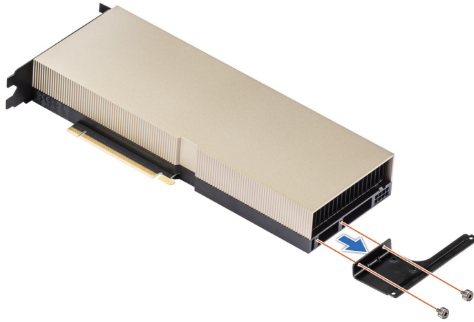
Figure 102. Removing the standard bracket with two screws
