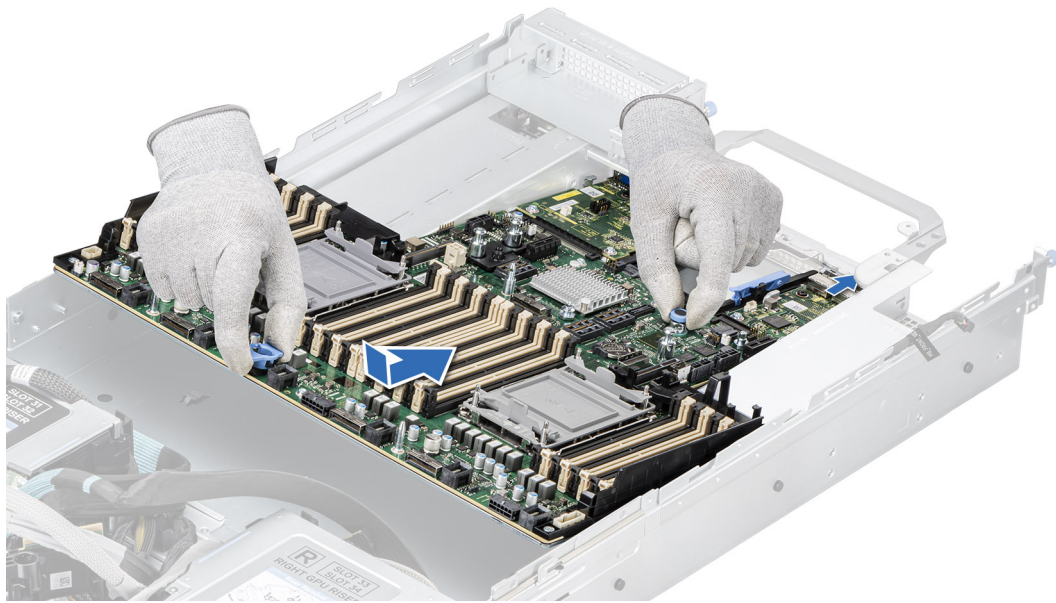
Figure 169. Installing the system board
