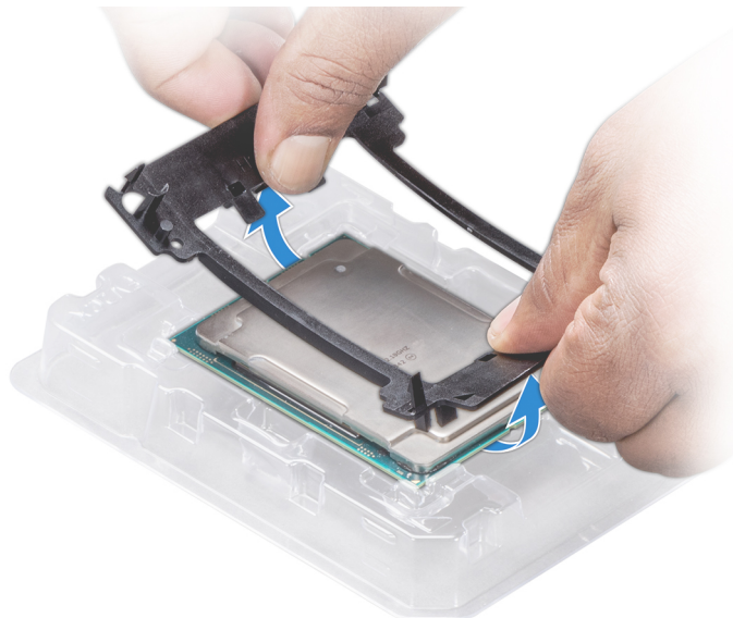
Figure 105. Removing the processor bracket
