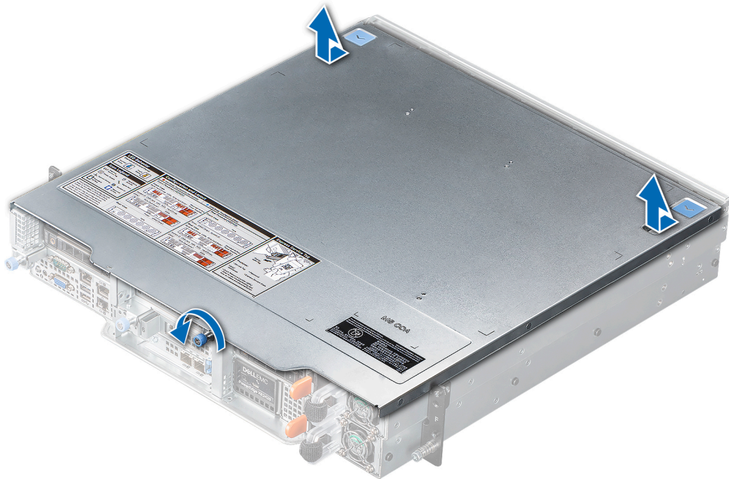
Figure 34. System cover removal
