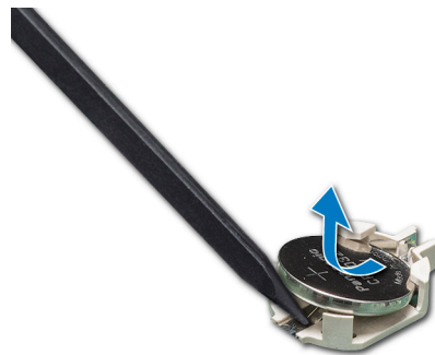
Figure 122. System battery removal
