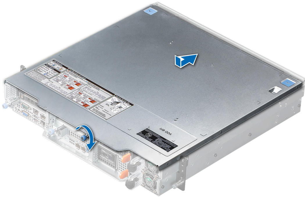
Figure 35. System cover installation
