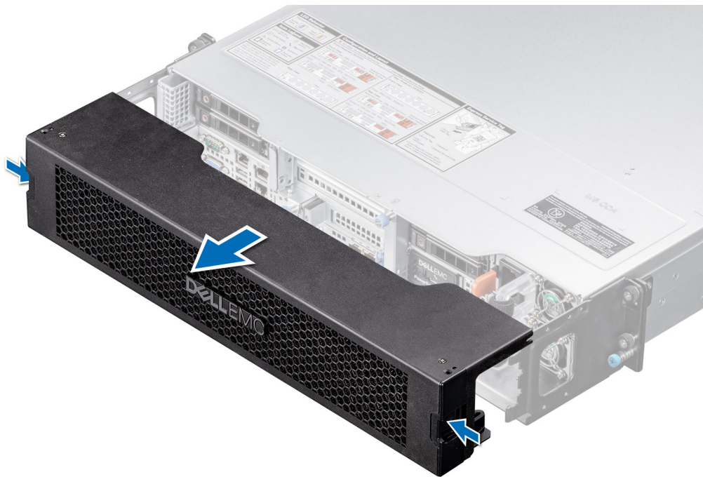
Figure 28. Front bezel cover removal
