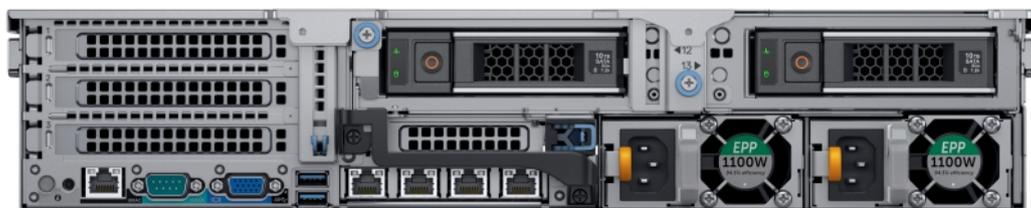
**Figure 12. Back view of 2 x 3.5 inch drive system**
