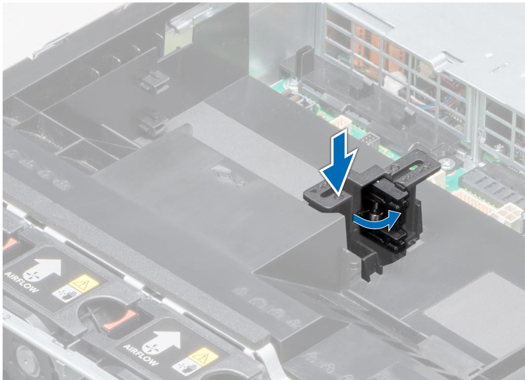
**Figure 78. Opening the PCIe card holder latch**
