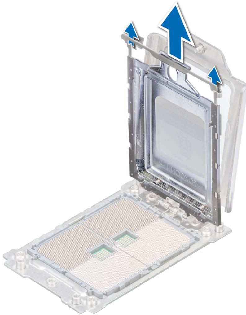
**Figure 73. Removing a processor blank**
