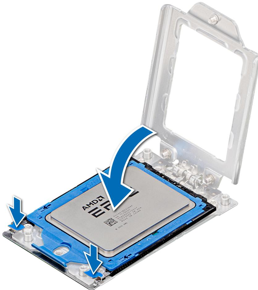
**Figure 75. Closing the processor socket frame**
