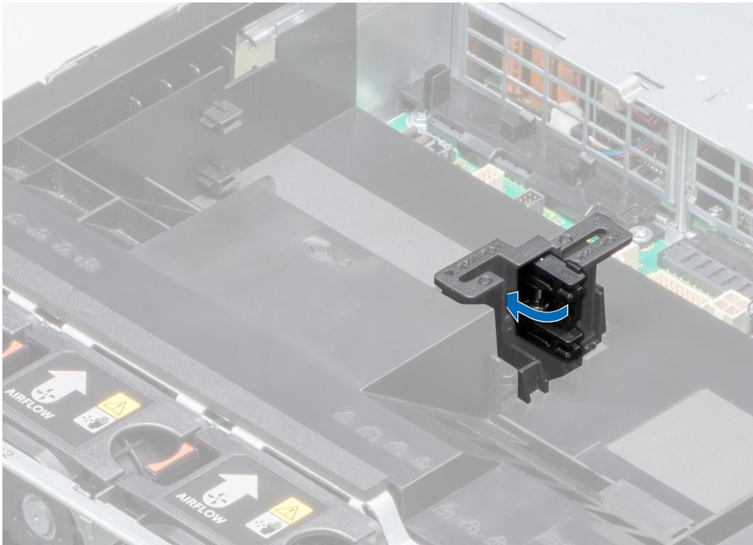
**Figure 79. Closing the PCIe card holder latch**
