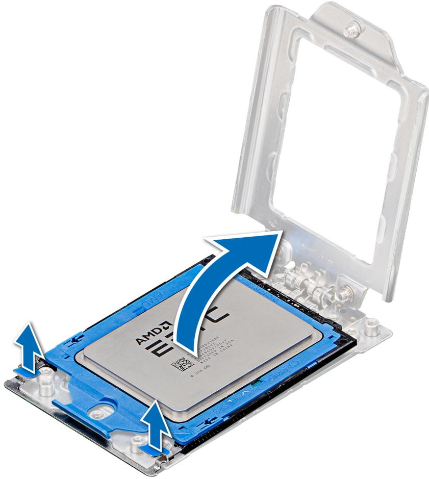
**Figure 70. Lifting the rail frame**
