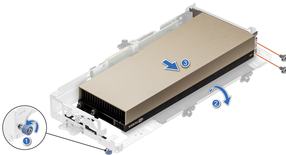
Figure 73. Removing a double-width, full-length GPU card from Riser 3A
