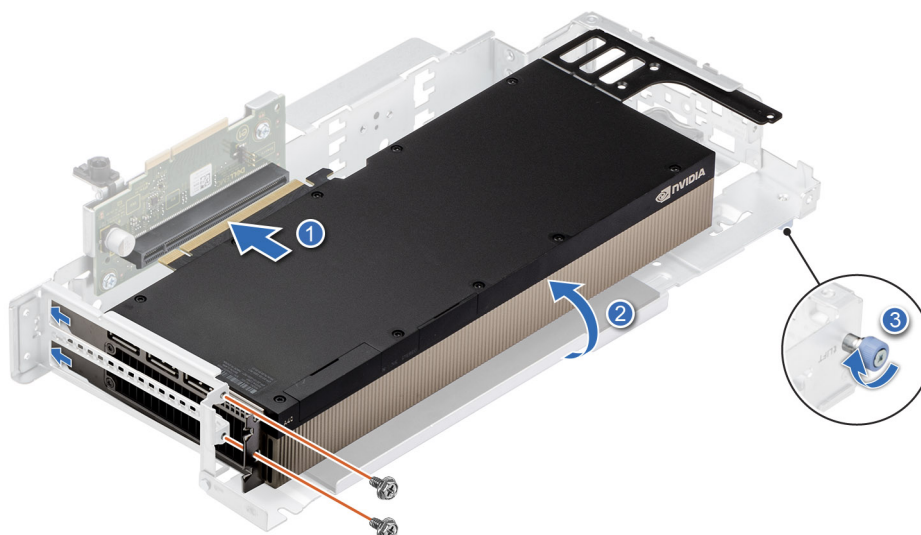
Figure 70. Installing a double-width, full-length GPU card into Riser 2A
