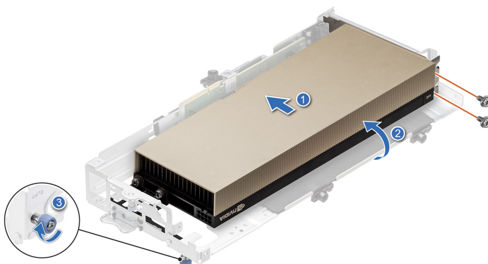
Figure 81. Installing a double-width, full-length GPU card into Riser 3A
