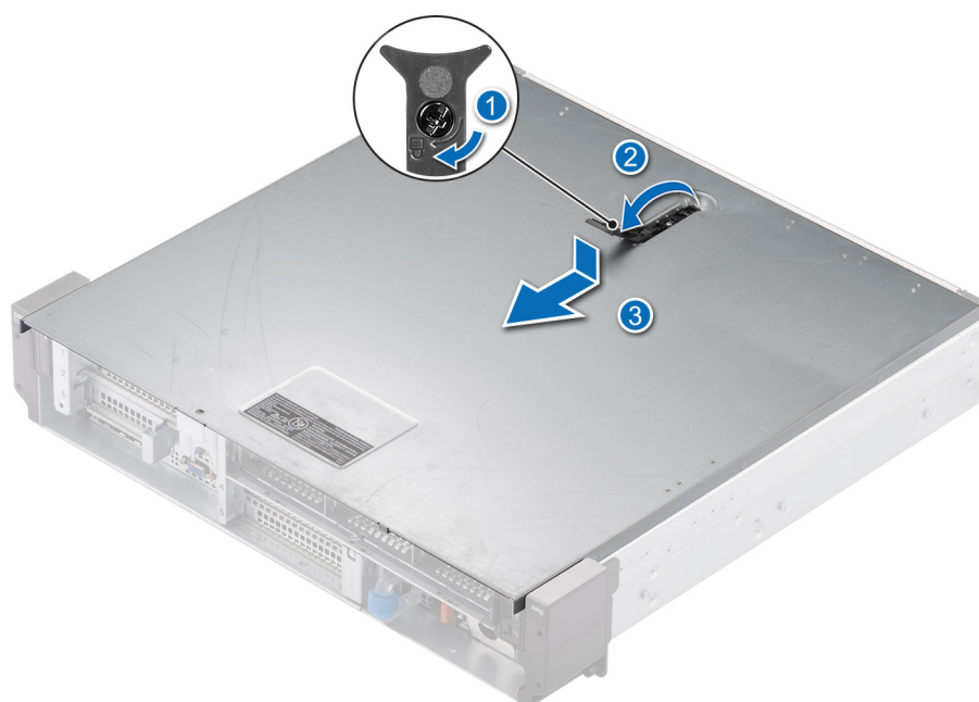
Figure 28. Removing the system cover for Front Accessed configuration
