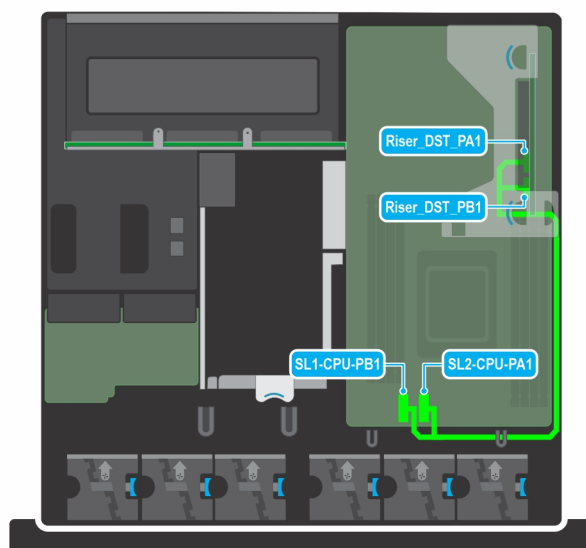
Figure 99. Riser 1A connecting on system board
