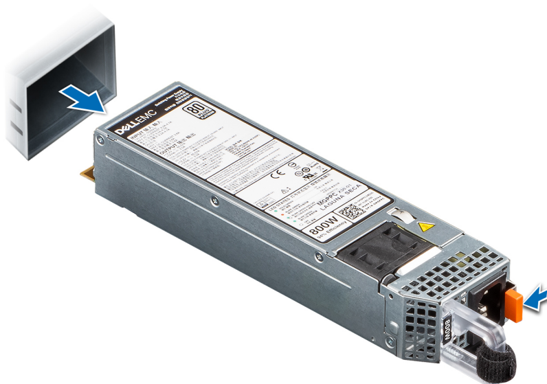
Figure 133. Removing a power supply unit
