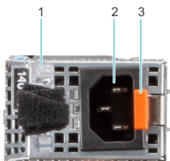
Figure 171. Rear Accessed configuration - AC PSU status indicator
