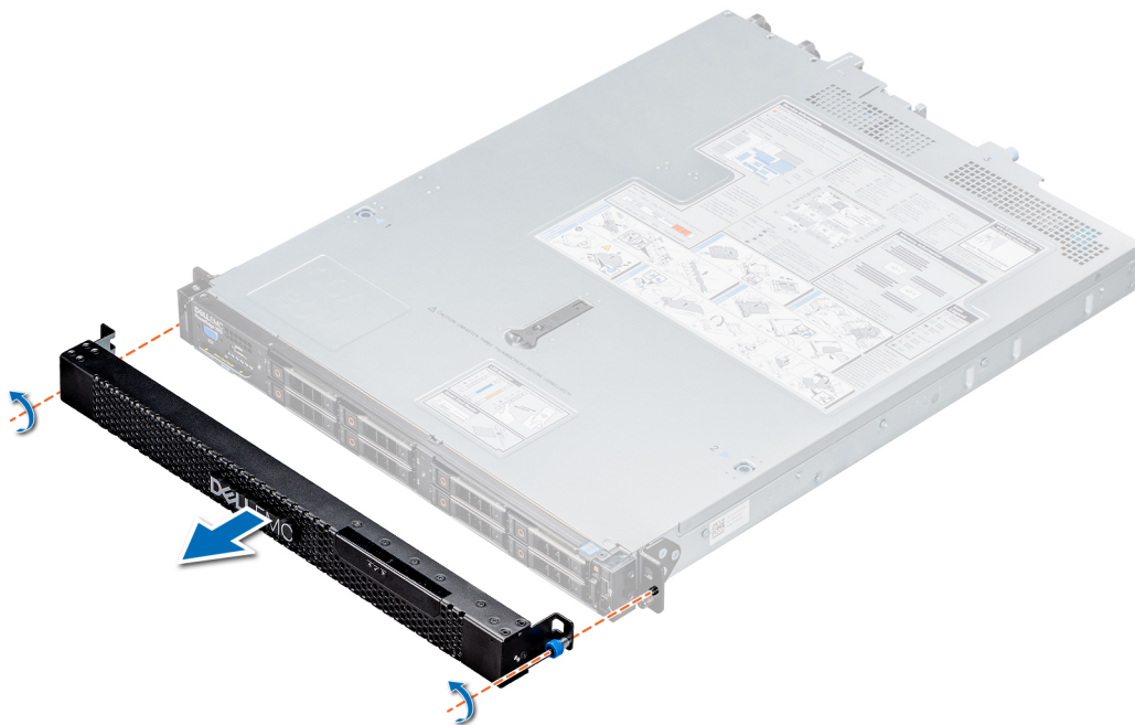
Figure 18. Removing the front bezel
