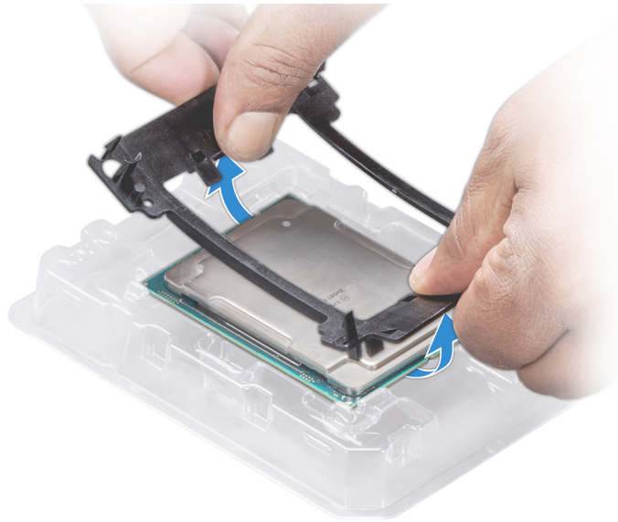
Figure 54. Removing the processor bracket
