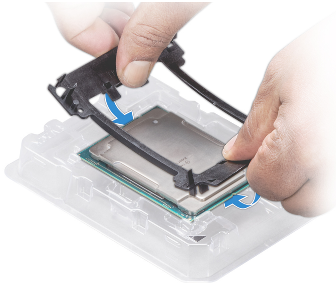
Figure 55. Installing the processor bracket
