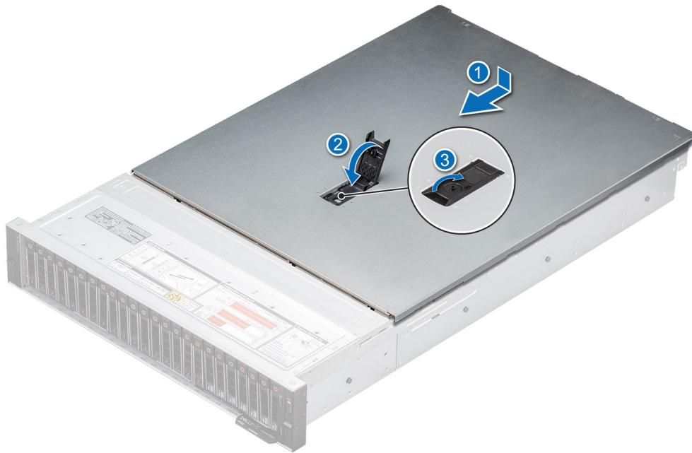
Figure 28. Installing the system cover
