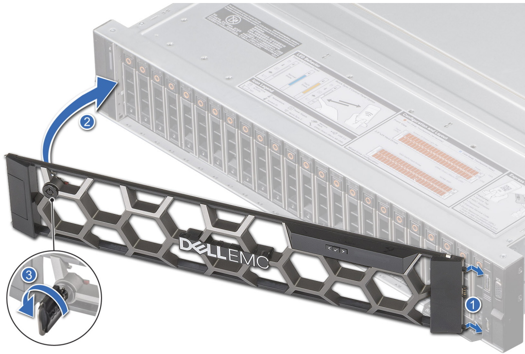
Figure 26. Installing the front bezel with the LCD panel
