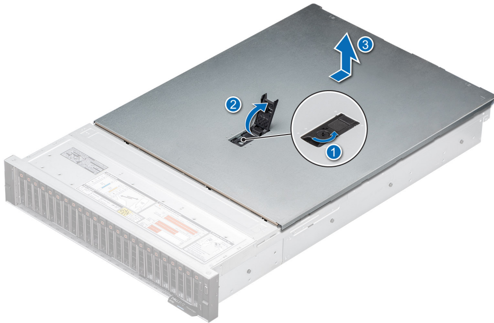
Figure 27. Removing the system cover
