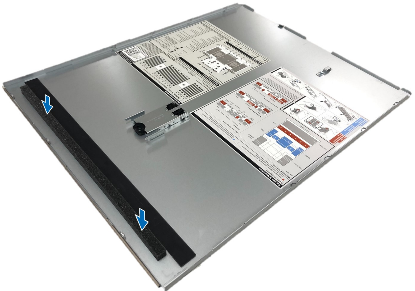
Figure 232. Installing Mylar foam on the system cover
