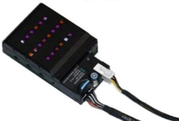
Figure 238. Connect power and signal cables to NVDIMM battery
