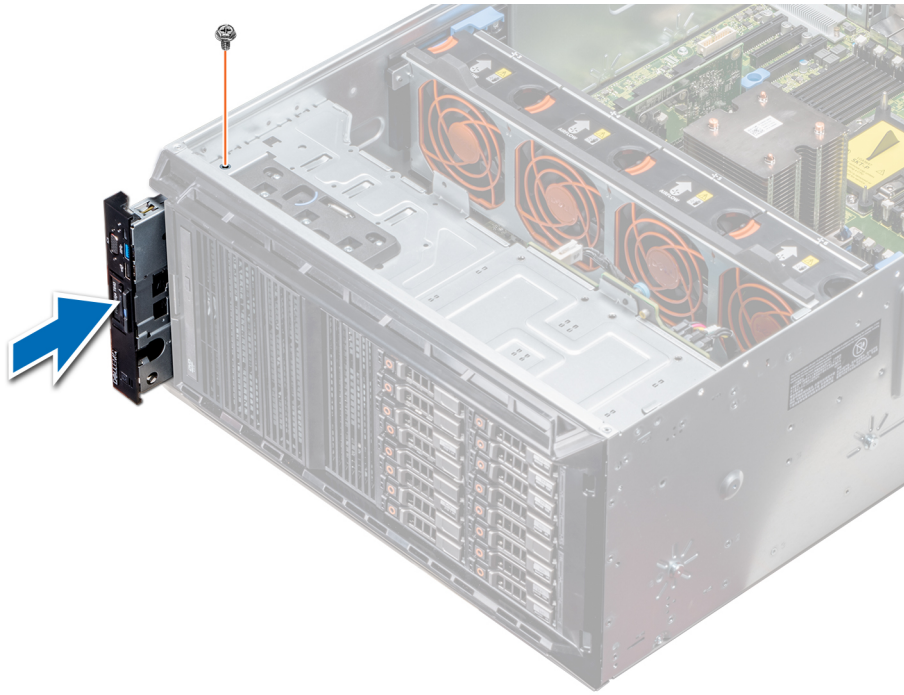
Figure 116. Installing the control panel assembly
