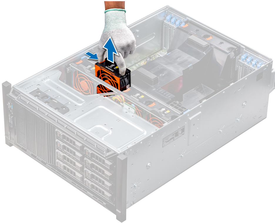
Figure 46. Removing a middle cooling fan
