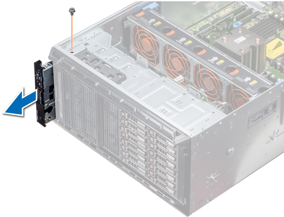
Figure 113. Removing the control panel assembly
