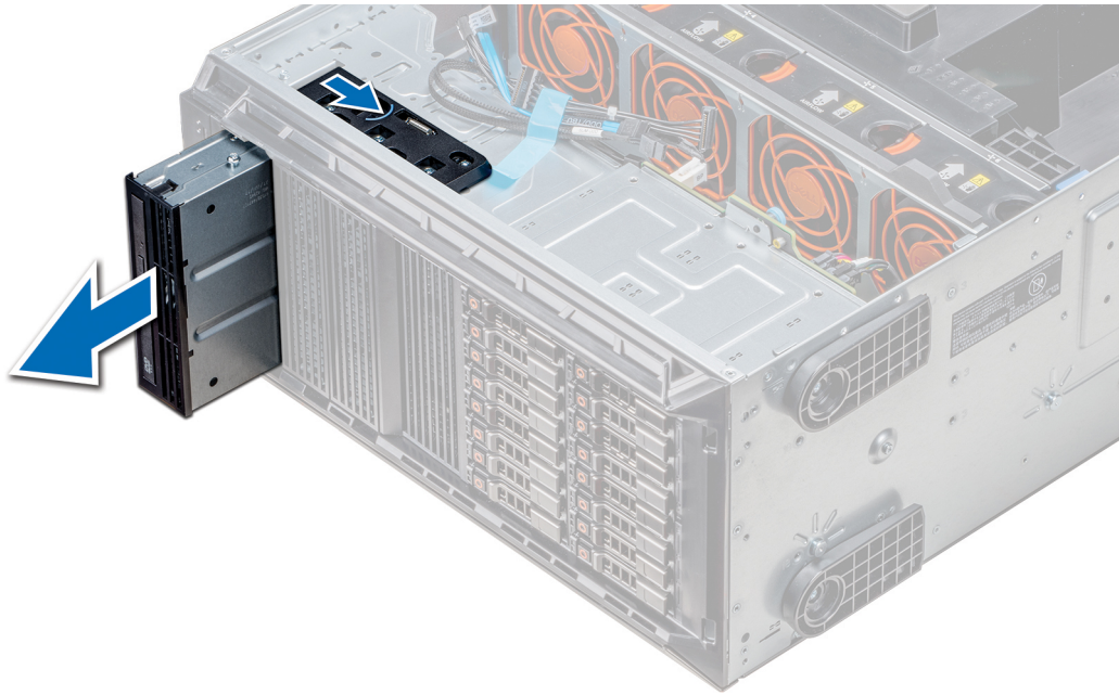
Figure 56. Removing the optical drive cage or tape drive
