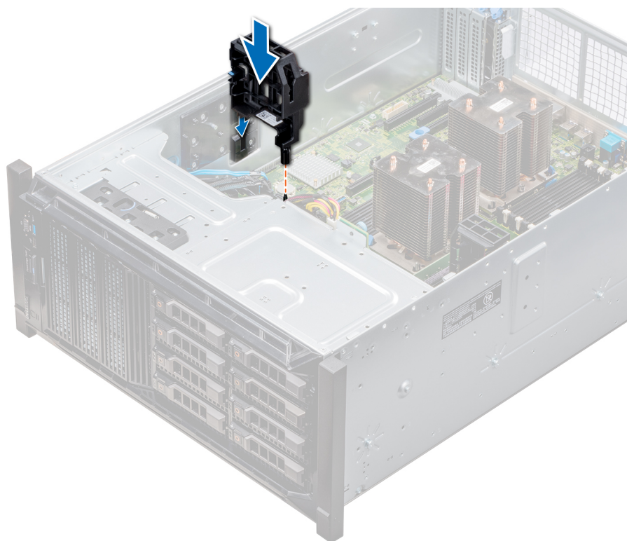
Figure 75. Installing the optional GPU card holder
