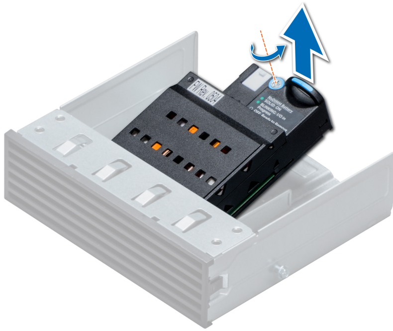
Figure 60. Removing the NVDIMM-N battery
