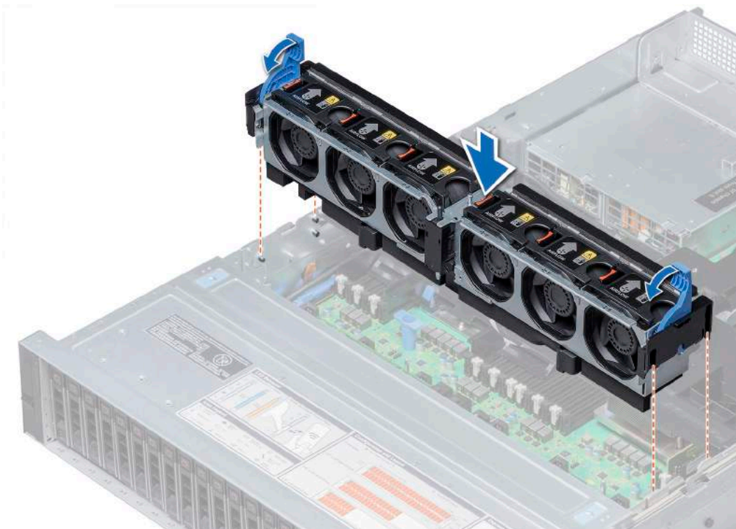
Figure 28. Installing the cooling fan assembly
