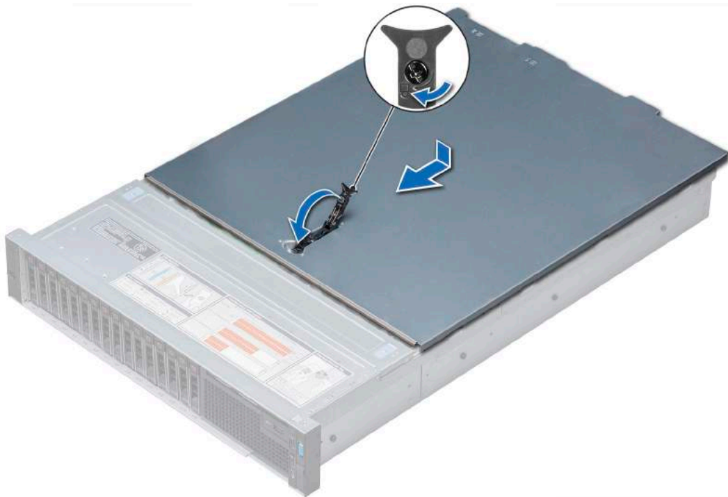
Figure 20. Installing system cover
