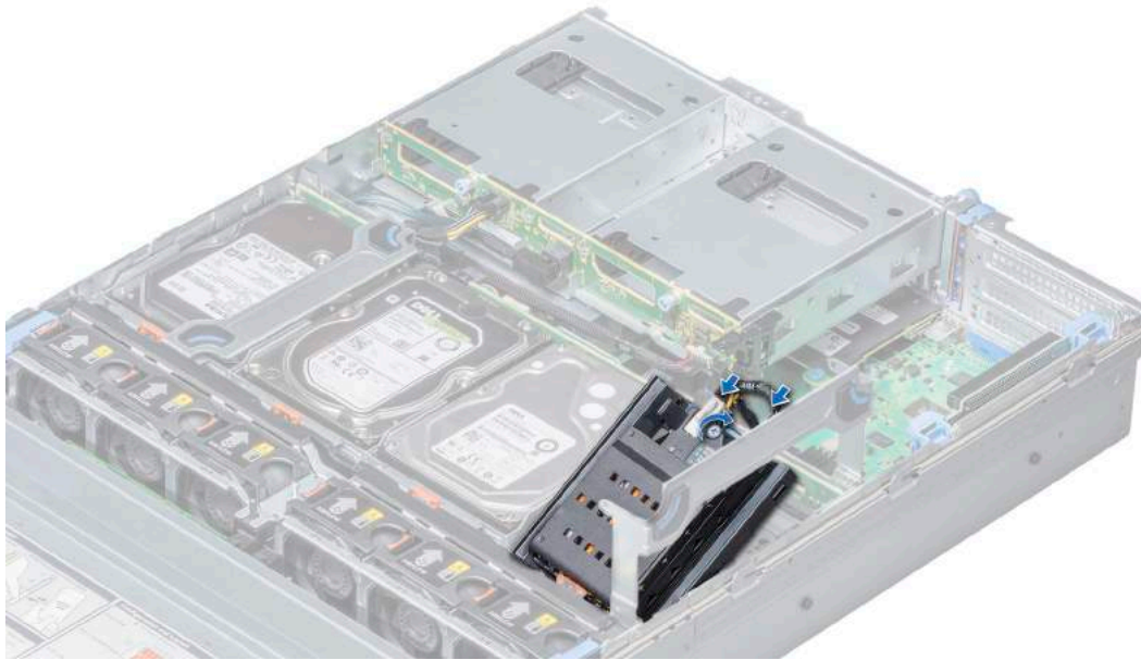
Figure 36. Installing NVDIMM-N battery into mid drive tray
