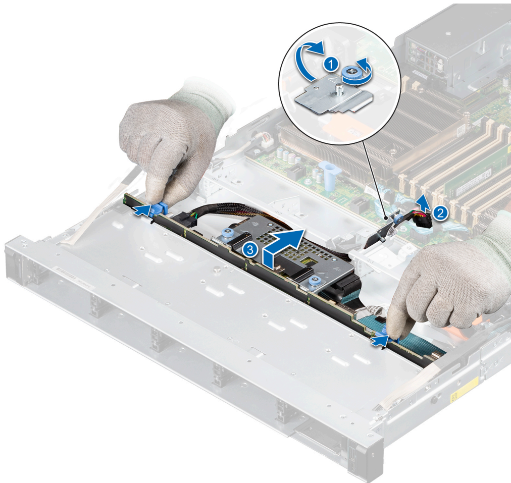
Figure 55. Removing the drive backplane
