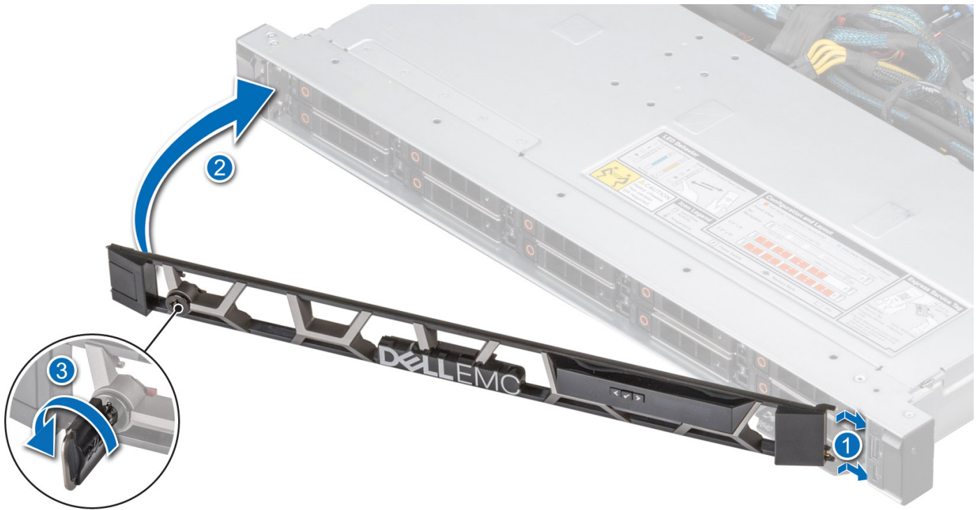
Figure 26. Installing the front bezel with the LCD panel
