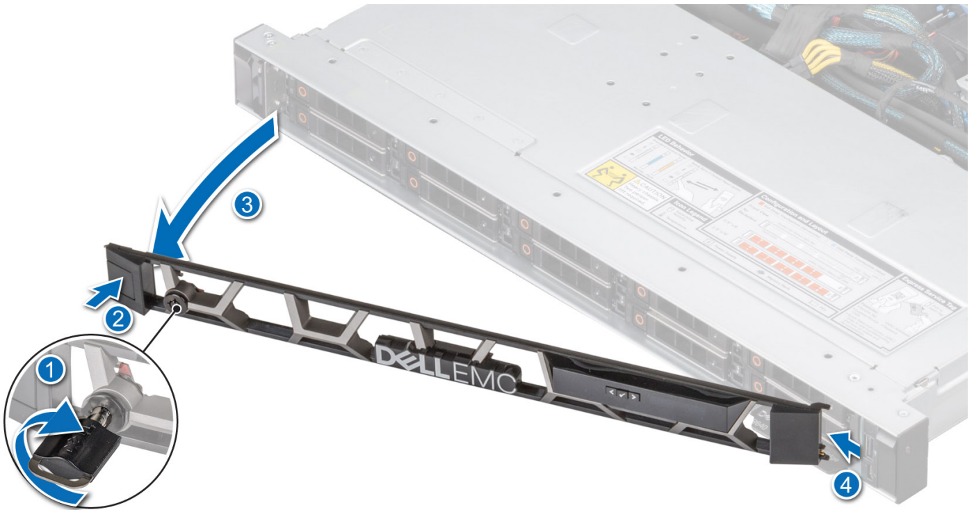
Figure 25. Removing the front bezel with the LCD panel
