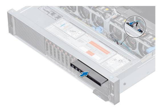
Figure 103. Installing optical drive
