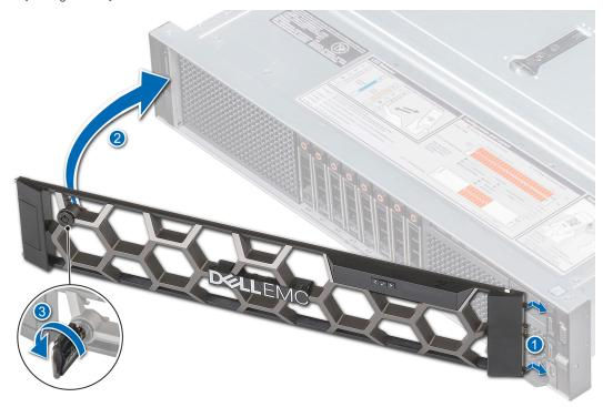
Figure 18. Installing the optional front bezel
