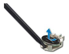
Figure 98. Removing system battery
