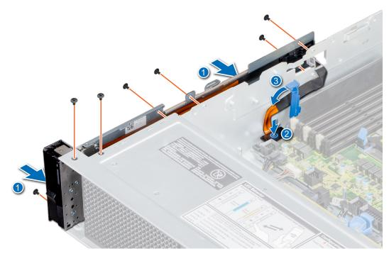
Figure 114. Installing left control panel
