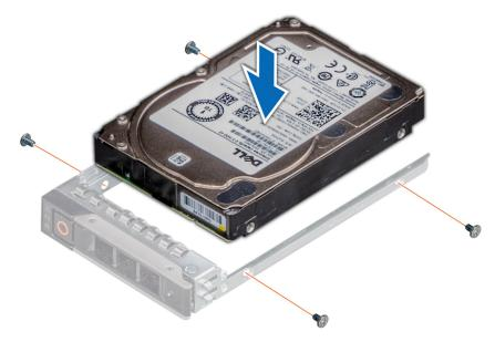
Figure 40. Installing a drive into the drive carrier
