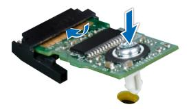
Figure 112. Installing the TPM
