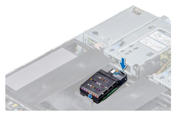
Figure 33. Installing NVDIMM-N battery into non-GPU air shroud
