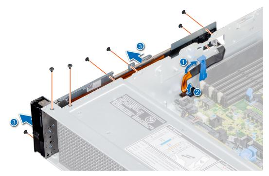
Figure 113. Removing left control panel
