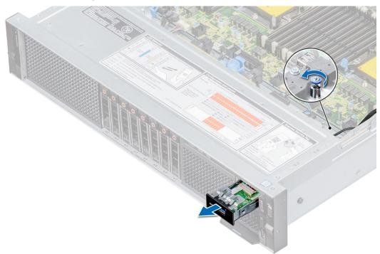
Figure 100. Removing USB 3.0 module
