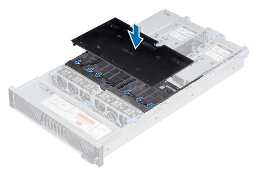
Figure 26. Installing the GPU air shroud cover
