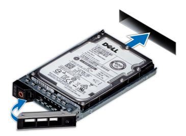
Figure 38. Installing a drive carrier
