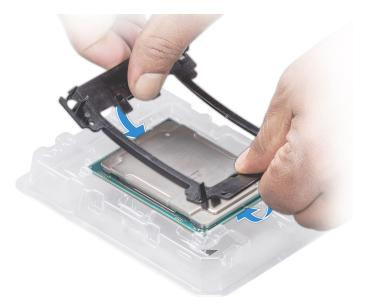
Figure 70. Installing the processor bracket
