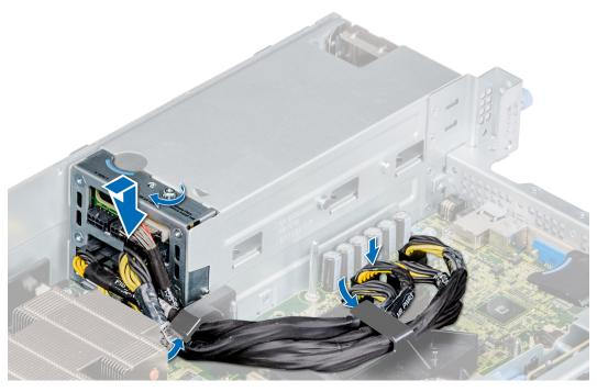
Figure 109. Installing power interposer board
