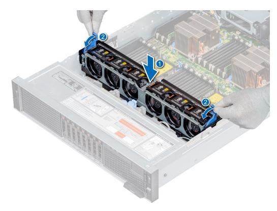
Figure 28. Installing the cooling fan assembly
