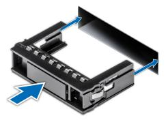
Figure 36. Installing a drive blank
