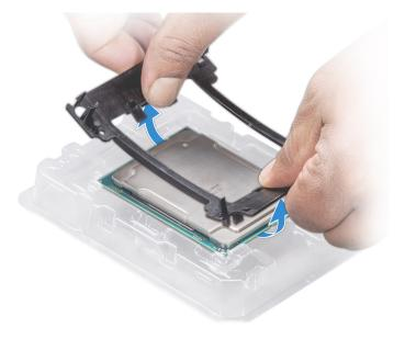
Figure 69. Removing the processor bracket
