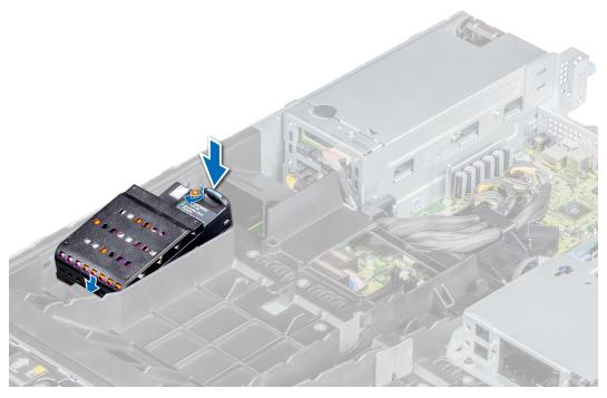
Figure 34. Installing NVDIMM-N battery into GPU air shroud
