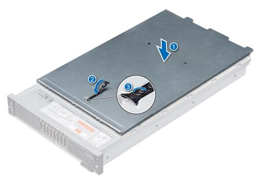
Figure 20. Installing system cover
