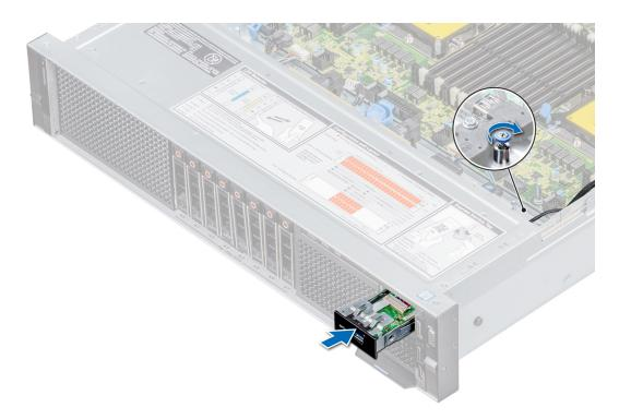
Figure 101. Installing USB 3.0 module
