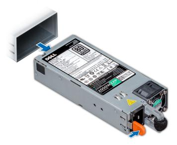
Figure 106. Removing power supply unit
