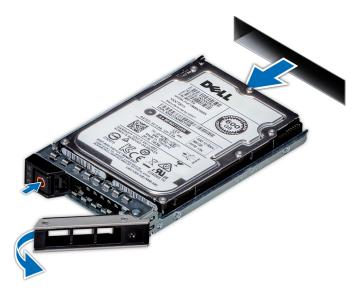
Figure 37. Removing a drive carrier
