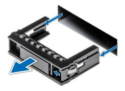
Figure 35. Removing a drive blank
